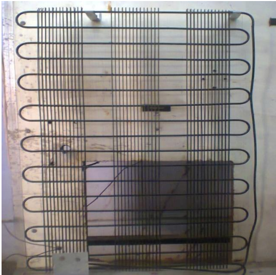
Figure 5.6: Finned-static air cooled condenser and specifications [RAC Lab, Thapar Uni.]
