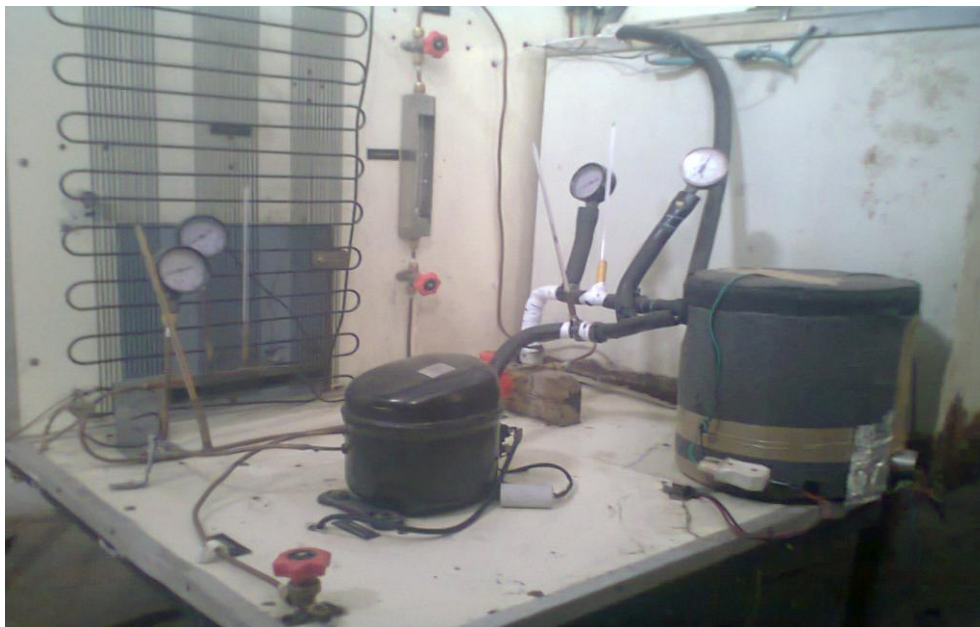
Figure 5.21: The domestic vapor compression refrigeration system setup in RAC Lab in Mechanical Engineering Department in Thapar University
