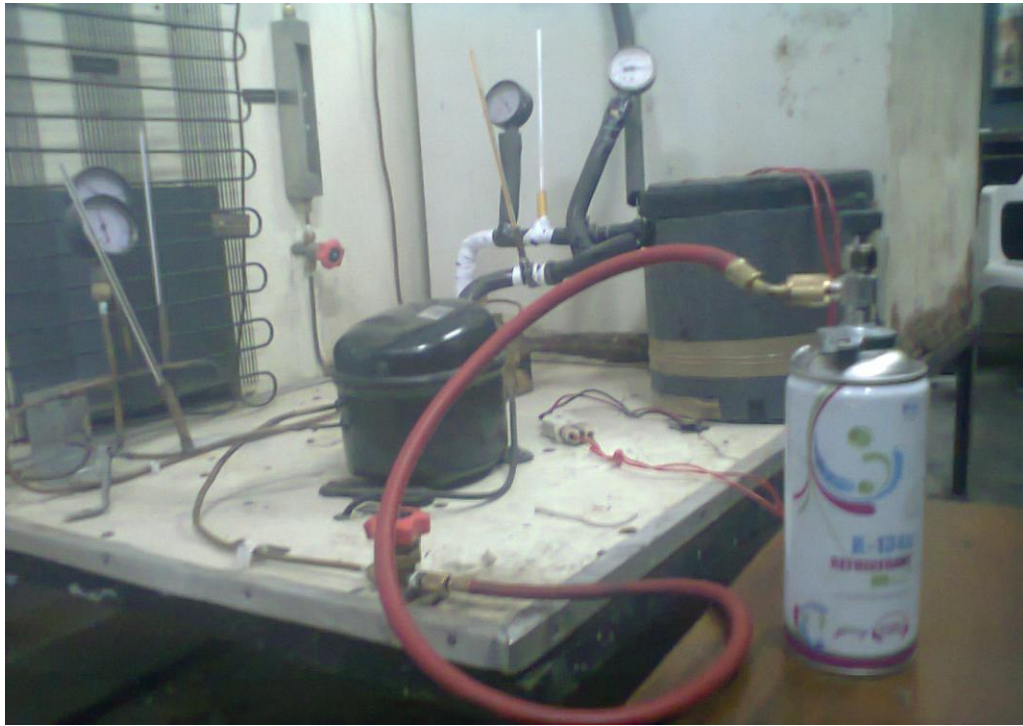
Figure 5.35: System charging nanorefrigerant (R134a+CuO) [RAC Lab, Thapar Uni.]
