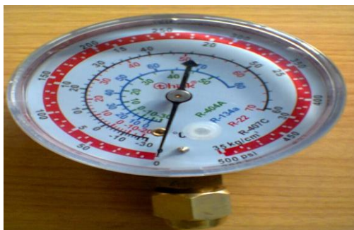
Figure 5.10: Pressure gauge for R-134a refrigerant [RAC Lab, Thapar Uni.]
