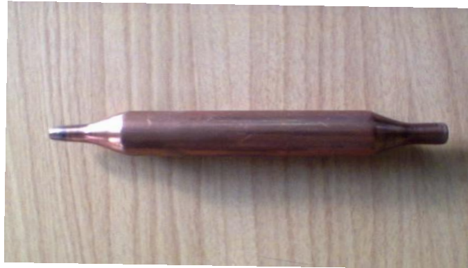
Figure 5.8: Filter dryer to remove moisture [RAC Lab, Thapar Uni.]
