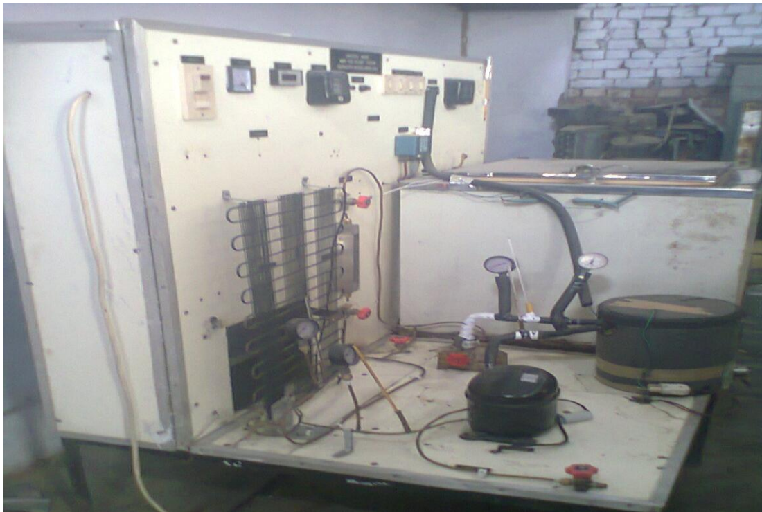
Figure 5.3: Experimental set-up components refrigeration system [RAC Lab, Thapar Uni.]
