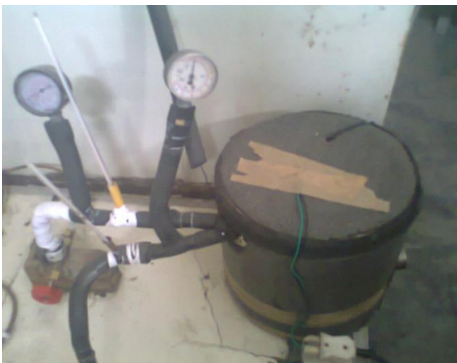
Figure 5.7: Coil type cylindrical evaporator and specifications [RAC Lab, Thapar Uni.]
