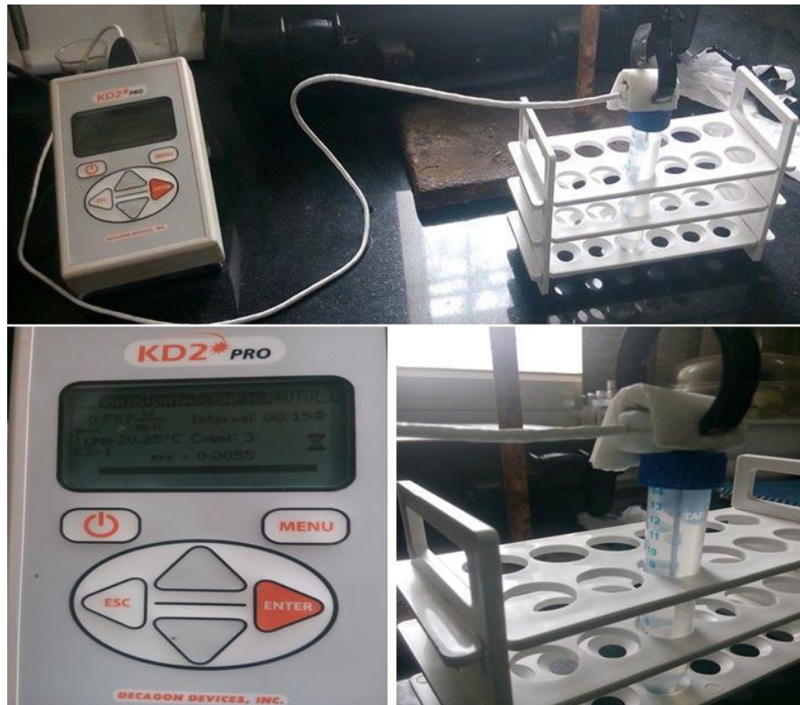
Fig 4.1.2 shows KD2 thermal properties analyzer set up with TIO2 nano-fluid
