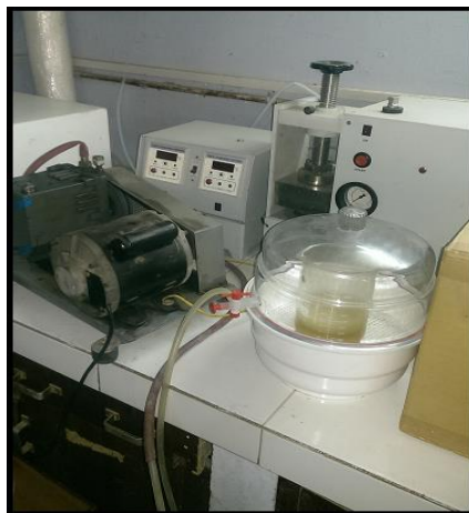
Figure 3.1 Desiccator with vacuum pump used in the present work.
