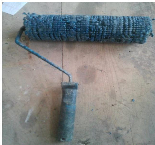
Fig-3.2 Roller For Spreading the Saturant of CFRP
