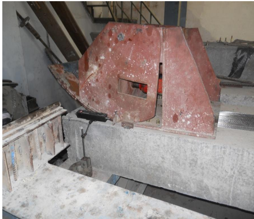
Fig-3.14 LVDT Used for Measuring the Elongation of CFRP
