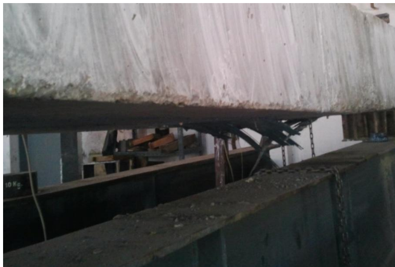
Fig-4.13 Crack Pattern of Retrofitted Beam with prestressing of 60% UTL of CFRP Sheet
