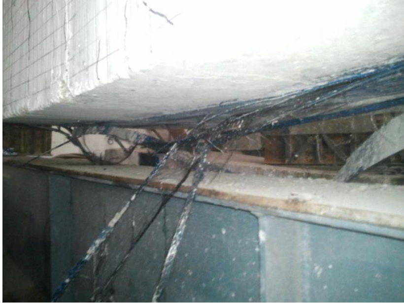
Fig- 4.18 Fiber Failure by Fracture of Retrofitted Beam with prestressing of 80% UTL of CFRP Sheet (01 RDB80)
