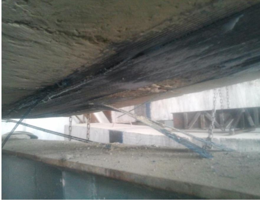
Fig-4.22 Fiber Failure by Fracture of Retrofitted Beam with prestressing of 80% UTL of CFRP Sheet (02 RDB80)
