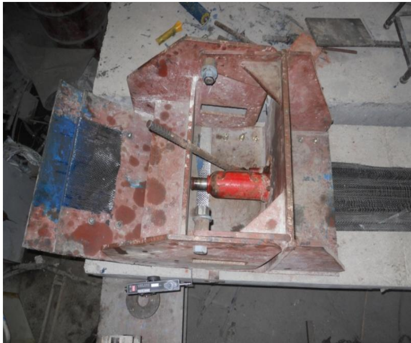
Fig -3.13 Prestressing of CFRP
