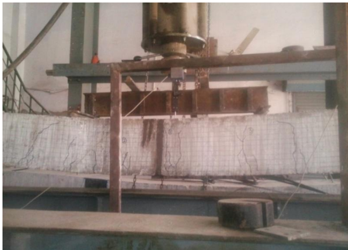
Fig- 4.21 Crack Pattern of Retrofitted Beam with prestressing of 80% UTL of CFRP Sheet (02 RDB80)
