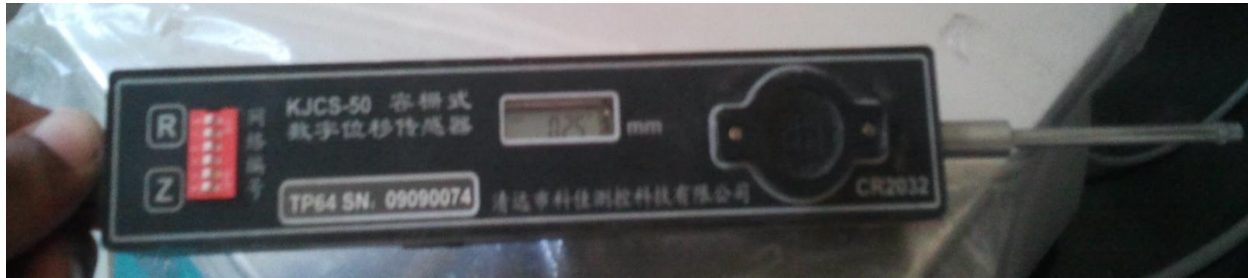
Fig-3.3 Liner Variable Differential Transducer
