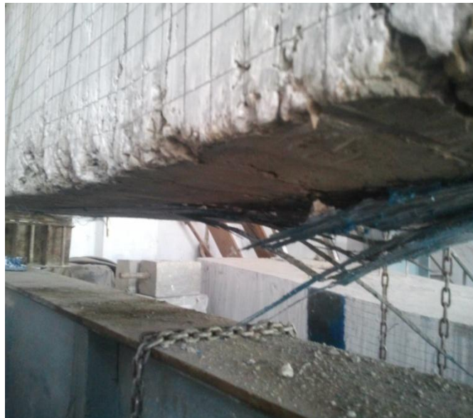
Fig- 4.10 Fiber Fracture 01 RDB60
