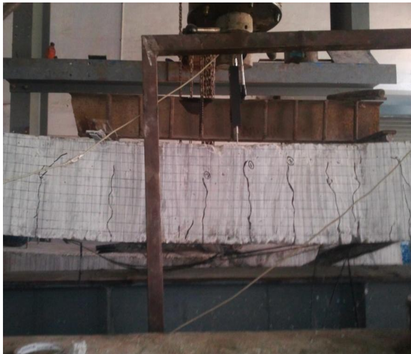
Fig- 4.17 Crack Pattern of Retrofitted Beam with prestressing of 80% UTL of CFRP Sheet (01 RDB80)
