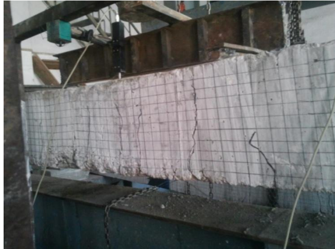
Fig –4.9 Crack Pattern of 01 RDB60
