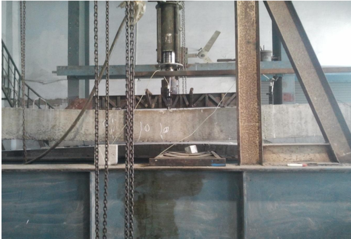
Fig-3.6 Two Point Loading System
