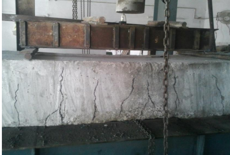
Fig-4.13 Crack Pattern of Retrofitted Beam with prestressing of 60% UTL of CFRP Sheet
