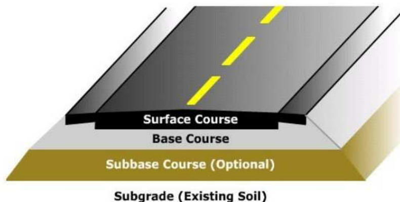
Figure 1.1: Components of Flexible Pavement Section
