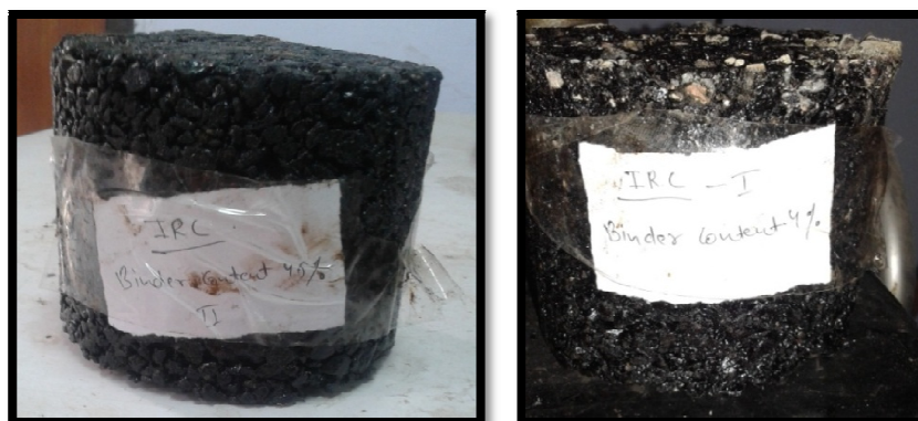
Figure 3.3: Bituminous Samples of MORTH gradation for 50 blows
