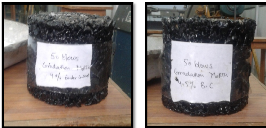
Figure 3.3: Bituminous Samples of MORTH gradation for 50 blows
