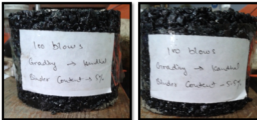
Figure 3.11: Bituminous Samples of Kandhal gradation for 100 blows
