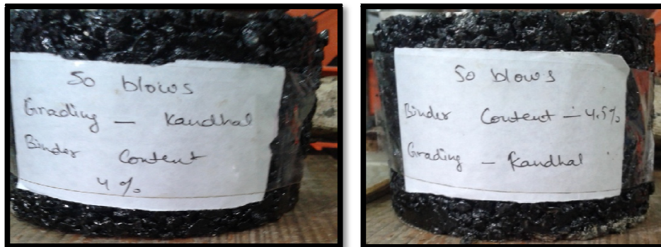
Figure 3.9: Bituminous Samples of Kandhal gradation for 50 blows
