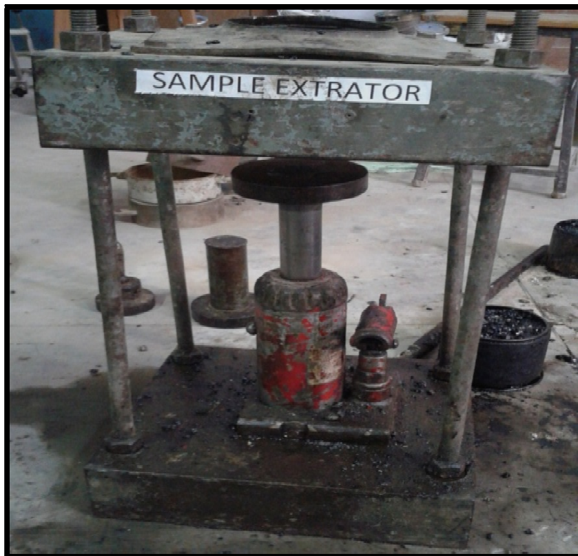
Figure 3.2: Sample Extractor for Marshall Specimen
