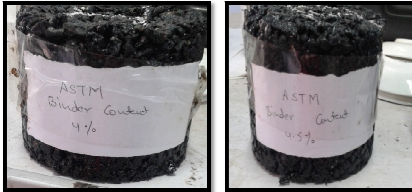
Figure 3.7: Bituminous Samples of ASTM gradation for 75 blows
