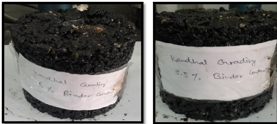
Figure 3.10: Bituminous Samples of Kandhal gradation for 75 blows
