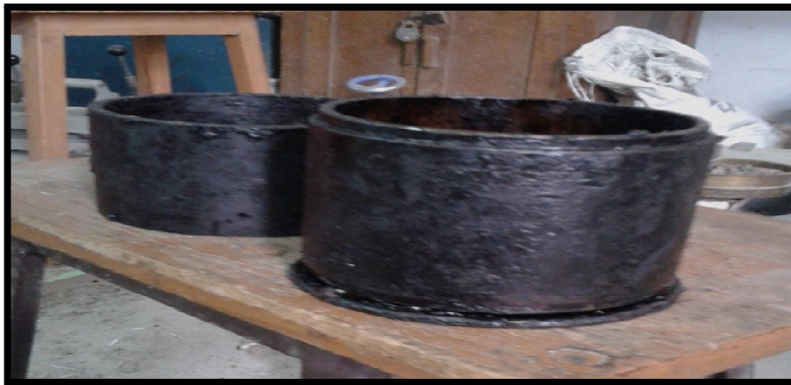
Figure 3.1: Mould Assembly of Marshall Test
