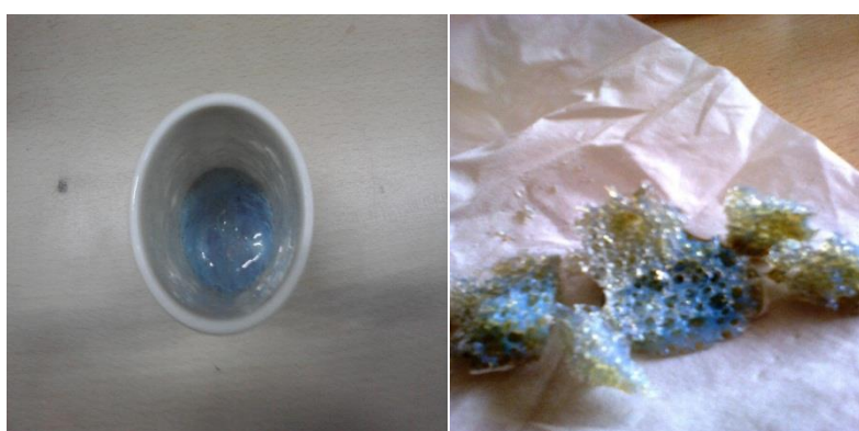
Figure 3.3 Molten mass in alumina crucible and glass sample.
