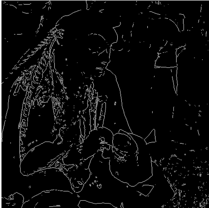
Figure 5.6(b) Sobel operator output
