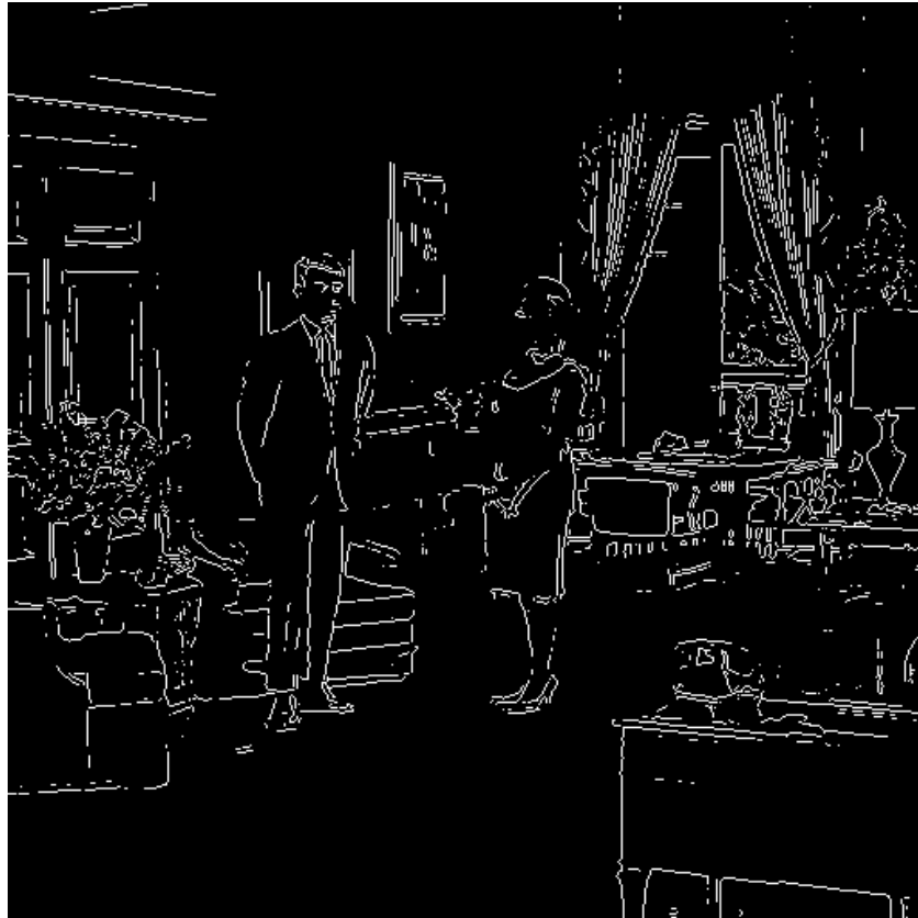
Figure 5.5(b) Sobel operator output
