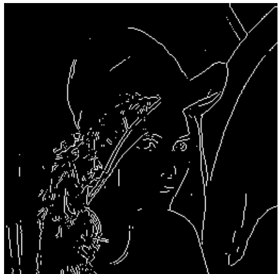
Figure 5.4(b) Sobel operator output
