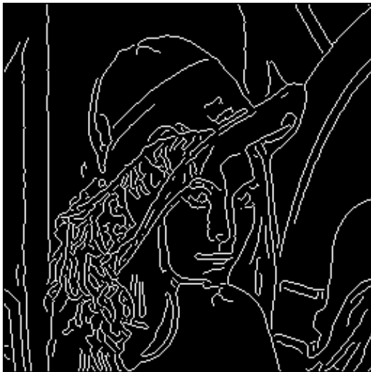
Figure 5.4(e) Canny operator output
