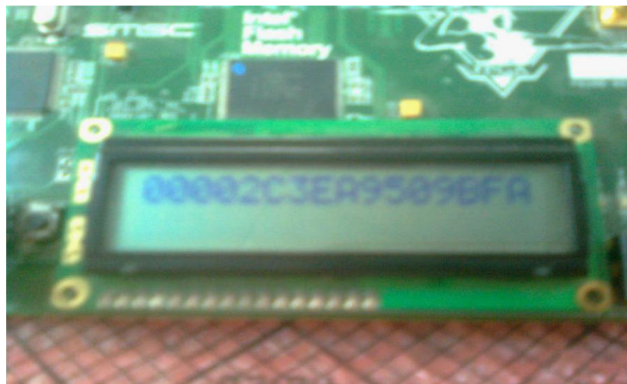
Figure 6.5: Output of 32X32 bit multiplier shown on LCD of Spartan kit
