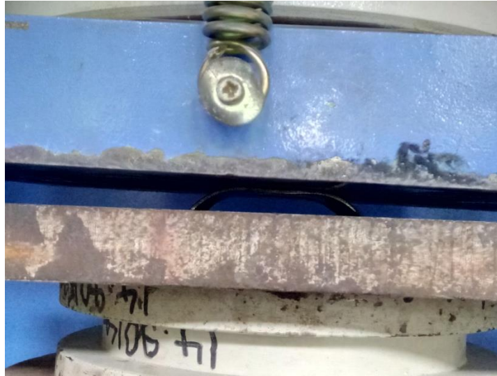
Figure 5.4 Deformation of curved sheet to flat
