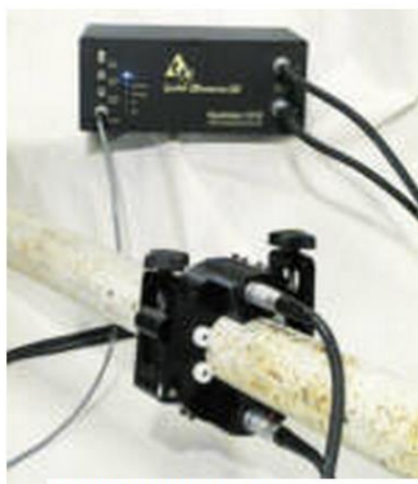
Guided Ultrasonics Ltd Wavemaker 16 instrument and transducer rings for 3 inch pipe
