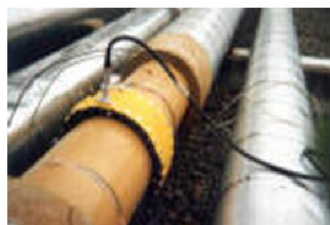
Flexible, pneumatically clamped transducer rings for larger diameter pipe
