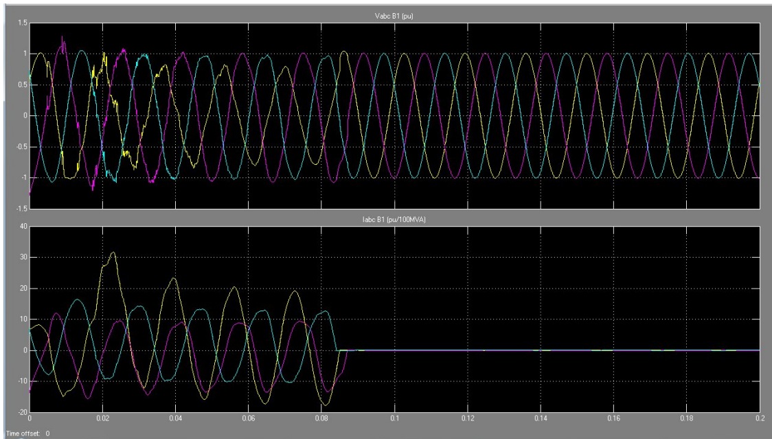
Fig 5.27 Three phase voltages and currents at B1
