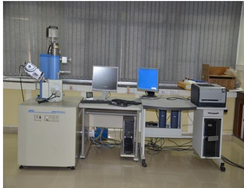
Fig 3.4 Scanning Electron Microscope used to study the surface morphology of GDC
