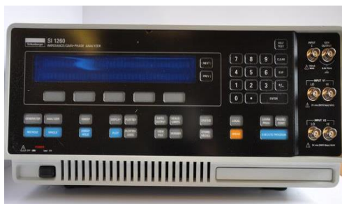
Fig 3.5 Impedance analyser used for dielectric measurement
