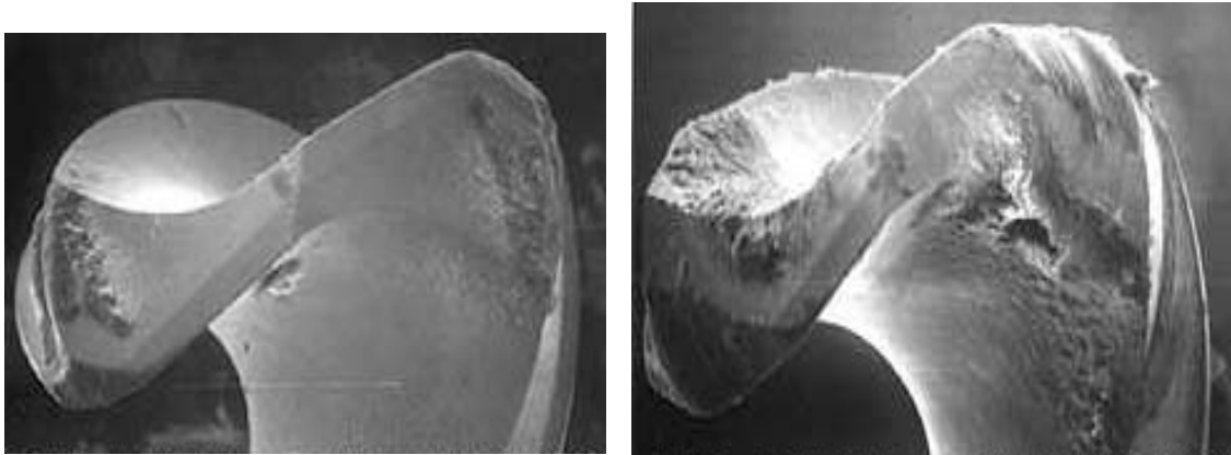
Figure 5.6 Influence of various speeds on tool wear (a) 510 (b) 3224 rpm respectively.
