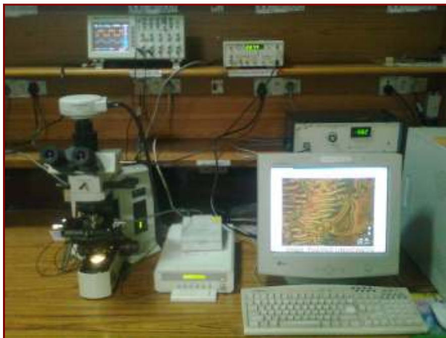
Fig. 2.4(b) Experimental set-up for the investigation of optical textures and electro-optic properties of chiral liquid crystal
