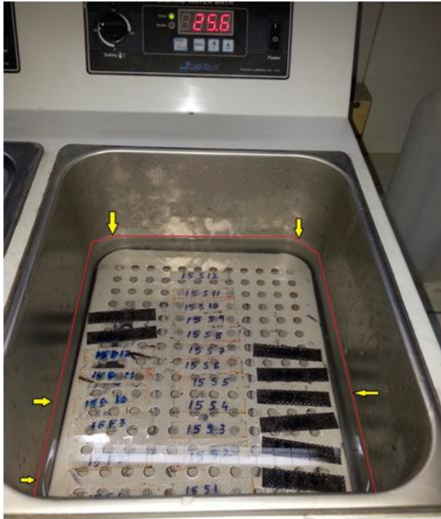
Figure 5.1: Hygrothermal aging of EP GFRP and CNT GFRP samples on immersion in water bath when studied in a seawater environment
