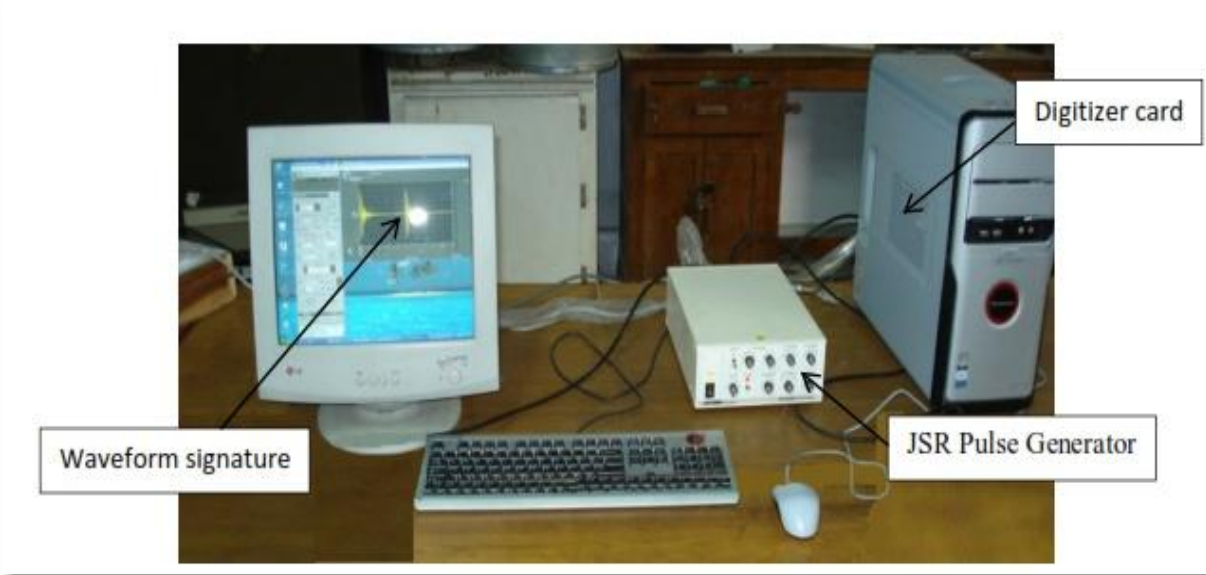
Figure 6.2: Ultrasonic testing set-up
