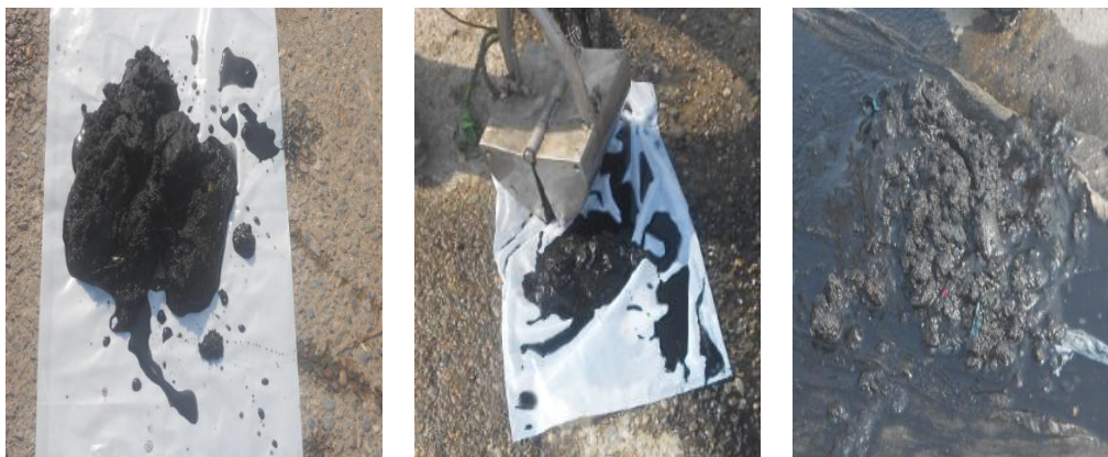
Figure 3.6: Collection of sediments using Ponar grab sampler
