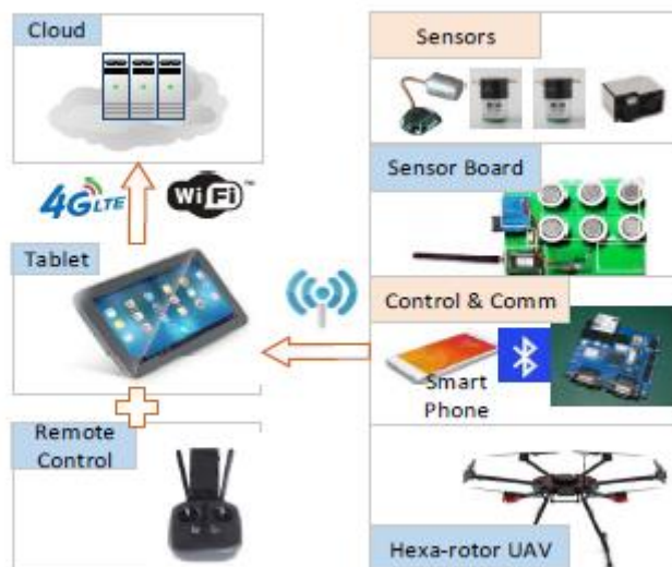
Figure 2.3 Architecture of IAQ monitoring system [27]
