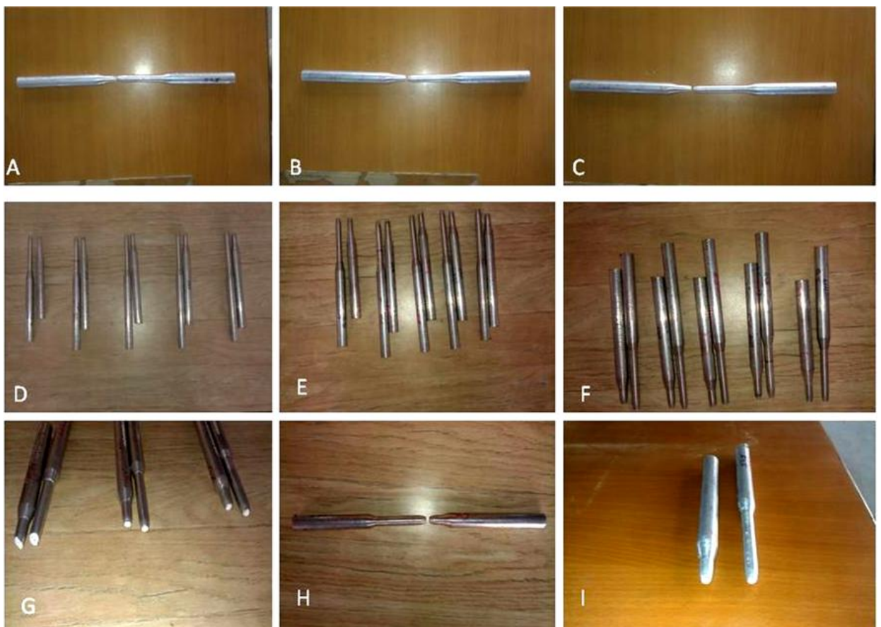
Fig.6.19 UTM Samples after break
