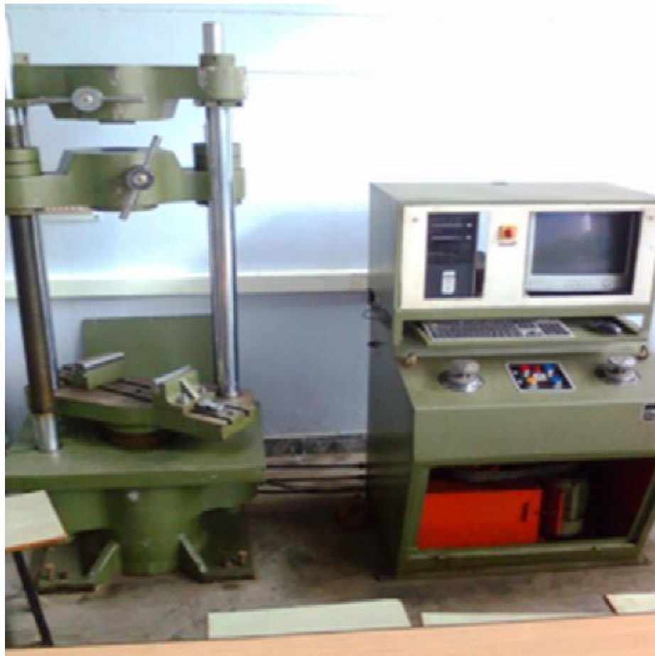
Fig.4.6 Universal Testing Machine [Courtesy by: CITCO. Chandigarh]
