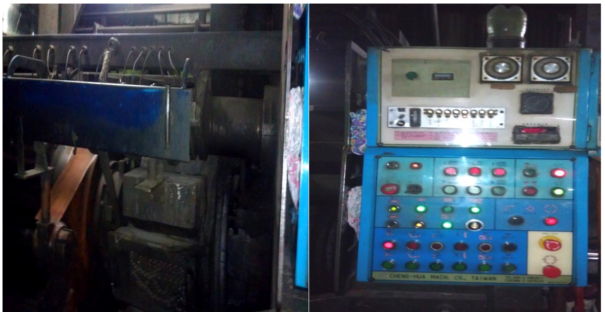
Fig.4.4 Horizontal Extrusion Press [Courtesy by: VALCO Steel Ltd. Chandigarh]
