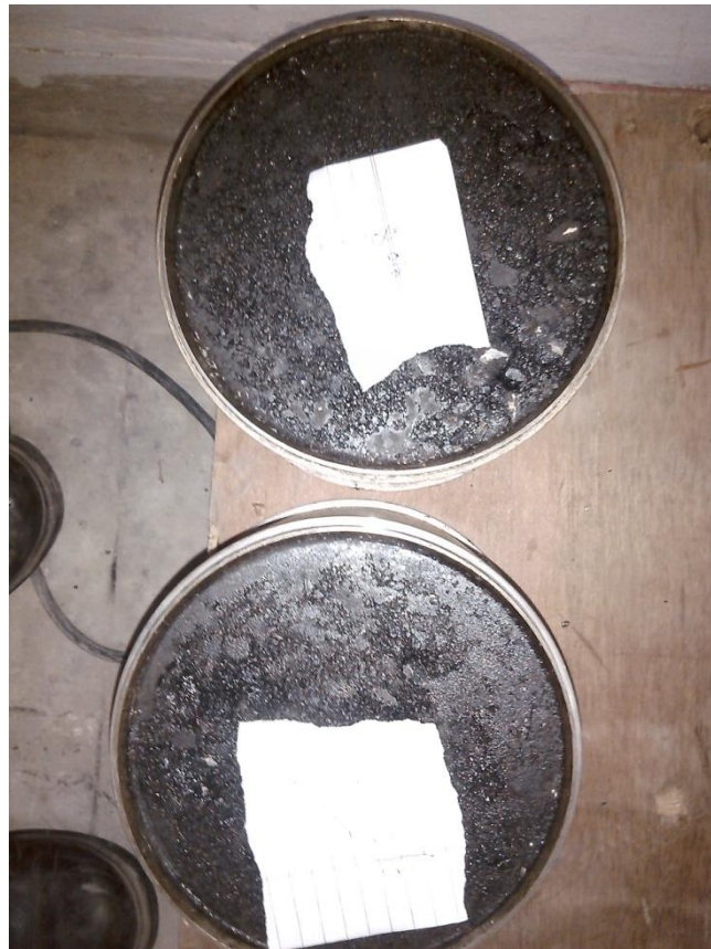
Plate-3.1 prepared specimens in a standard mould
