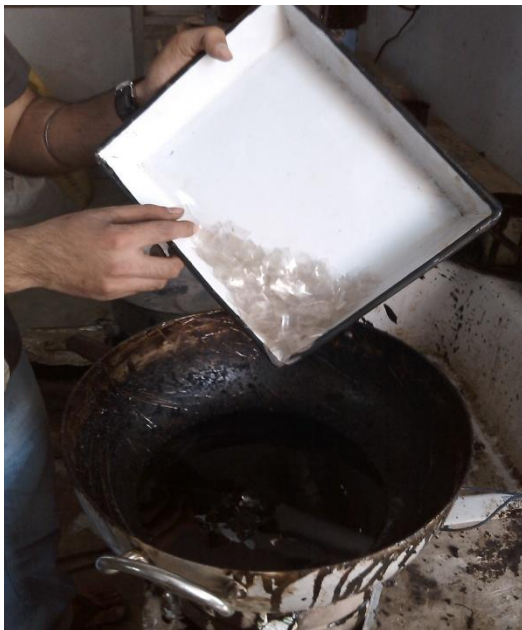
Plate 4.3 Mixing of Waste Bottle Pieces with Bitumen
