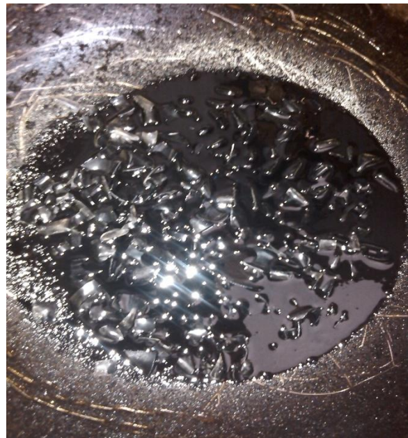
Plate 4.3 Mixing of Waste Bottle Pieces with Bitumen
