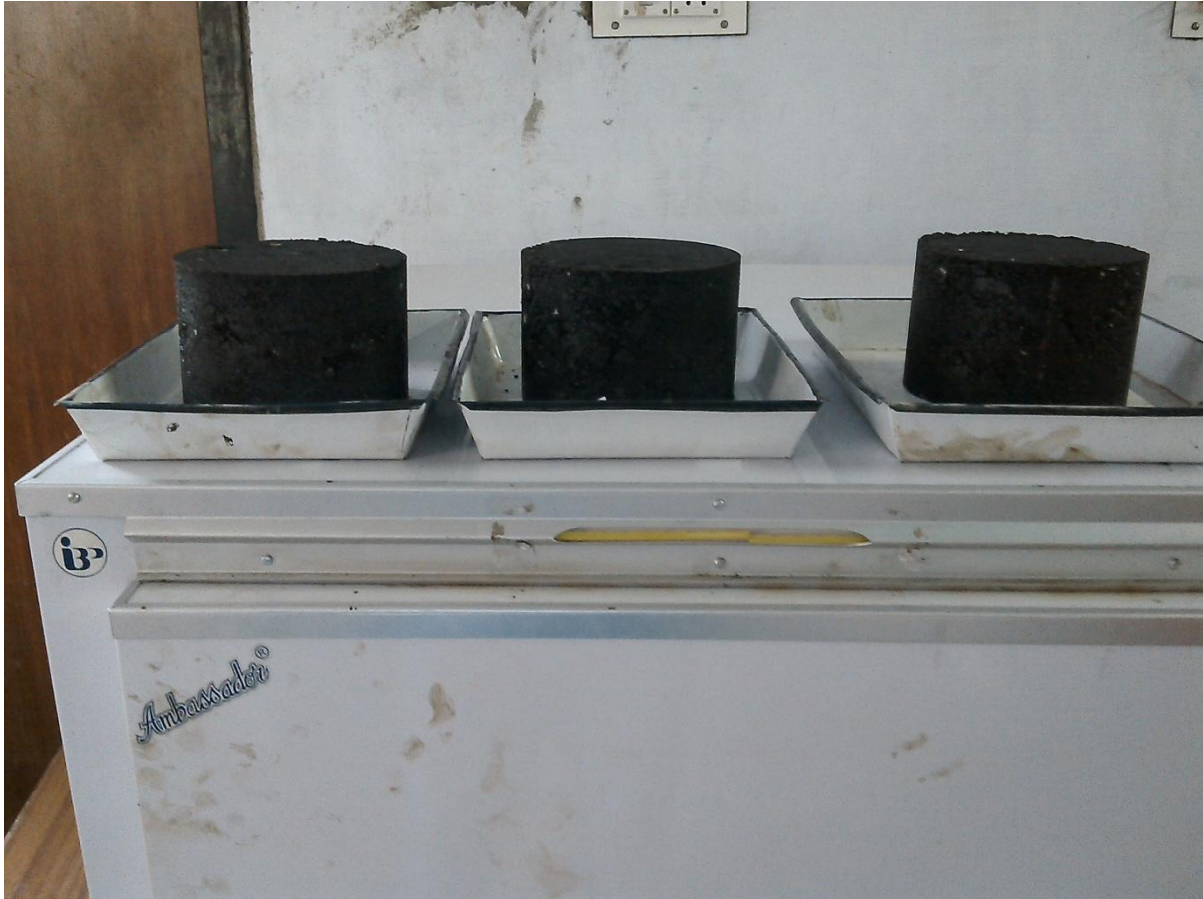
Plate 3.3-Samlpes Extracted from Marshalls Mould
