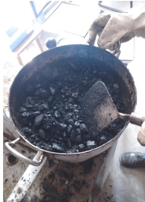
Plate 4.5 Mixing of Bitumen in Aggregate
