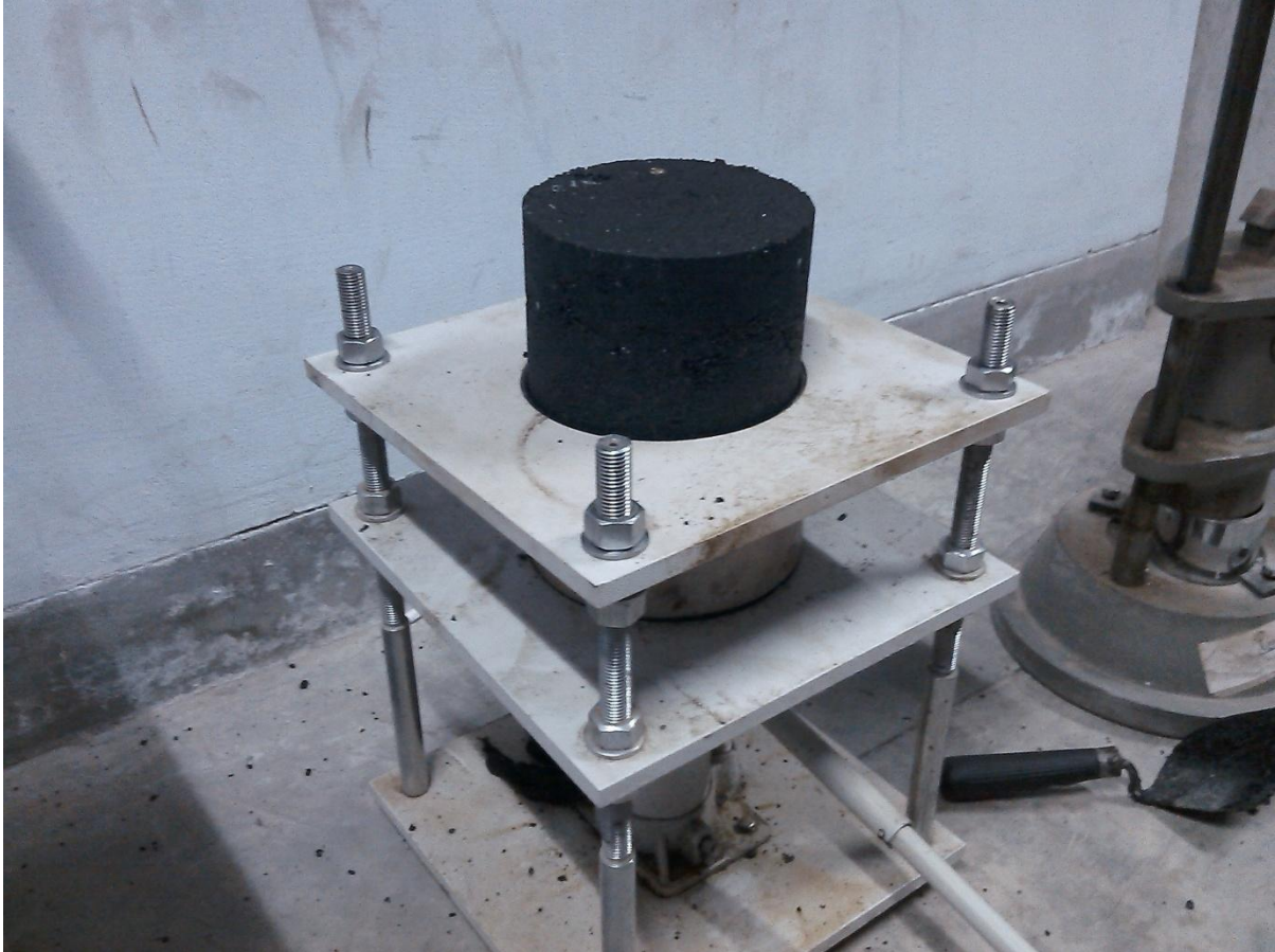
Plate 3.2 Sample Extraction from Extractor
