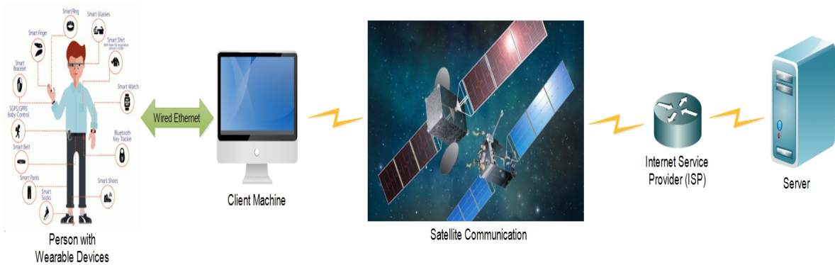
Figure 1.4: Communication Model in Sensors Network using Satellite
