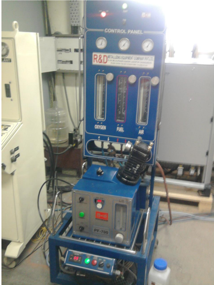
Figure 3.4 HVOF coating apparatus
