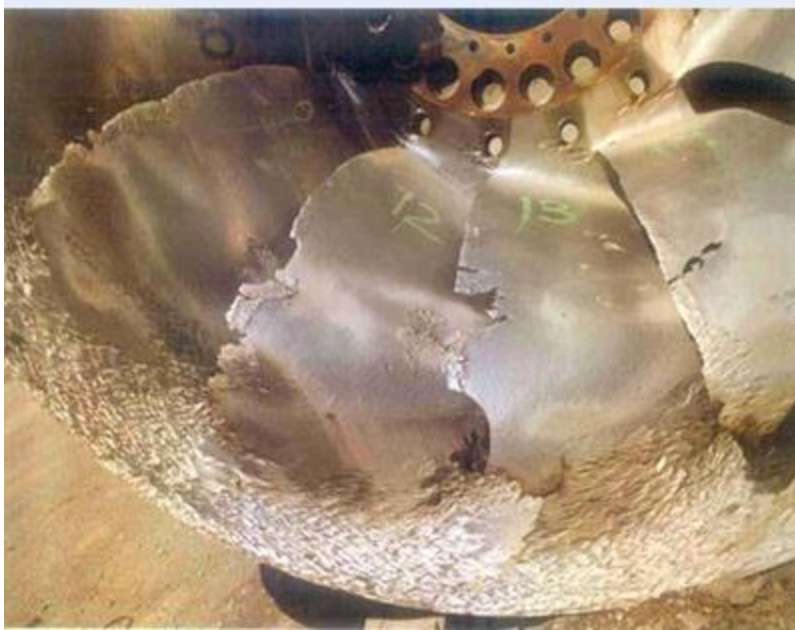
Figure 1.3 Eroded blades at Salal & BairaSiul Power Stations [NHPC]
