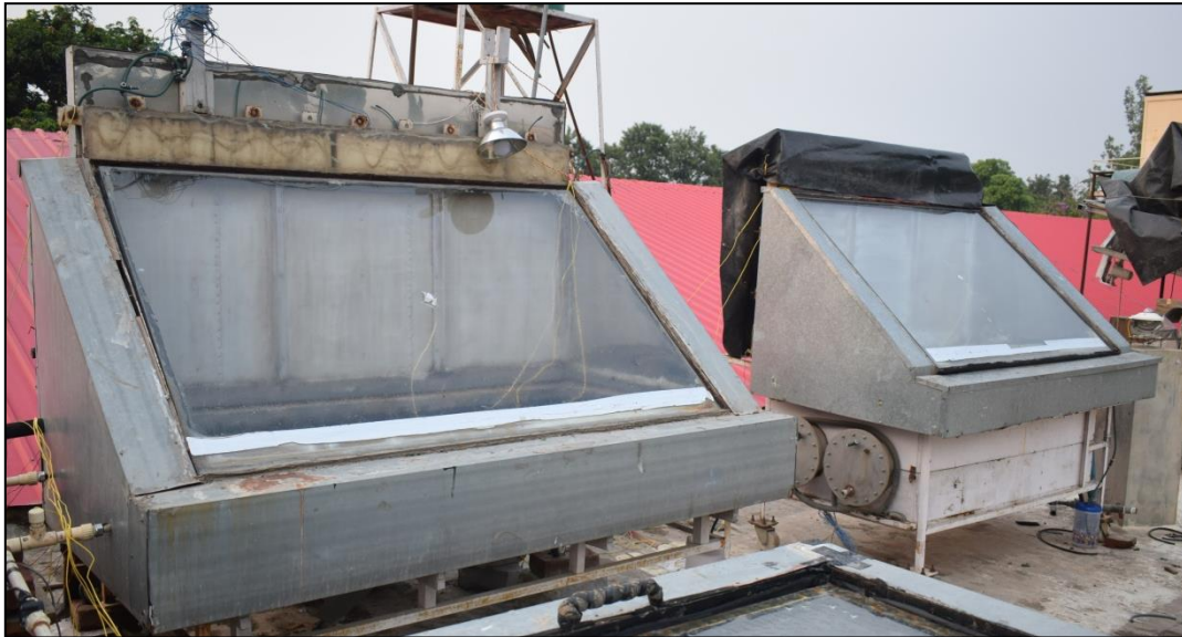
Fig 3.2. Experimental setup of single slope solar still.
