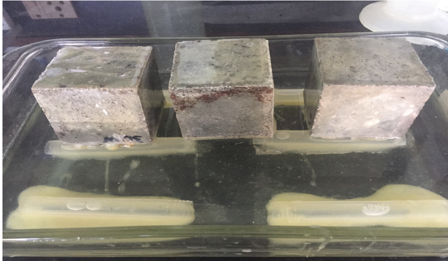
Fig. 3.8 Permeability analysis of motar cubes in a water tray
