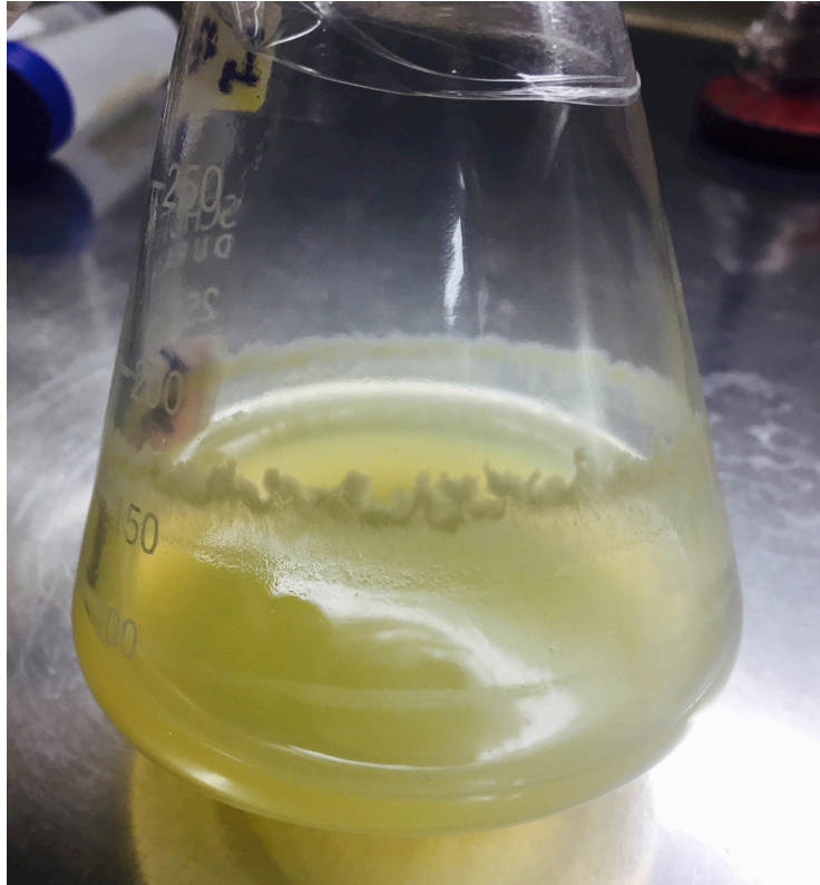
Fig. 3.4. Precipitates of \text{CaCO}_3 crystals along the walls as well as at bottom of flasks inoculated with PP9
