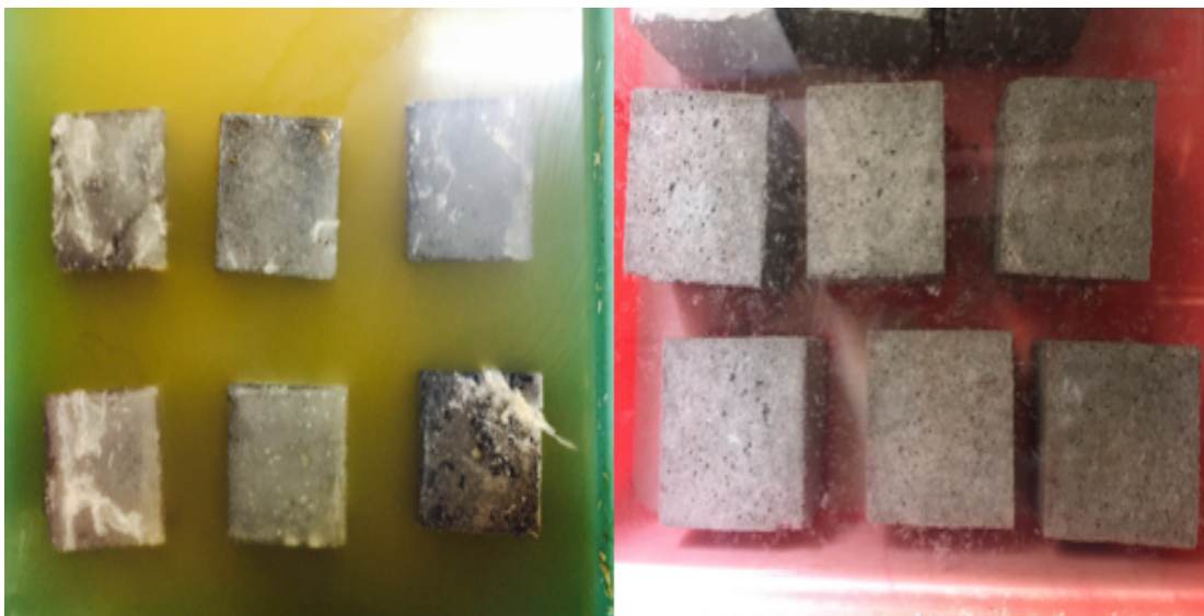
Fig. 3.6. Curing of cement motar cubes in NBU medium and water as specified in table 3.3
