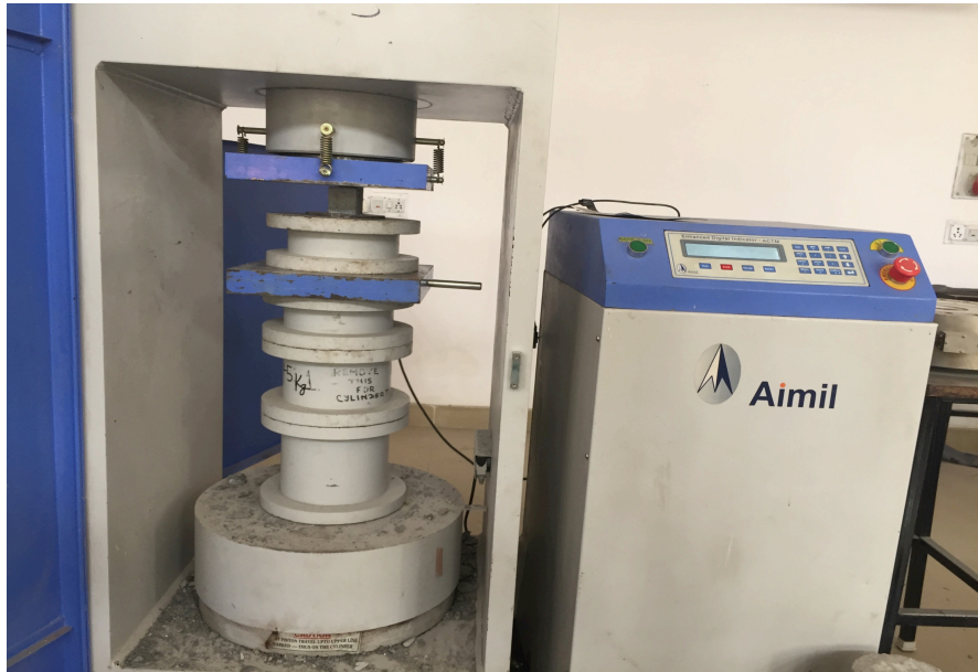
Fig. 3.7. Digital compression testing machine to test cube strength
