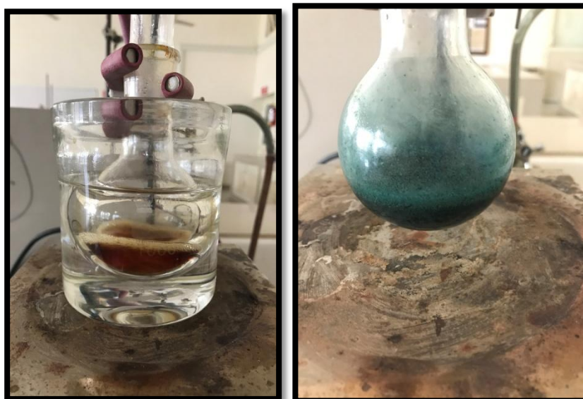
Figure 3.12: Change of colour from red – orange to blue due to addition of Copper perchlorate salt
