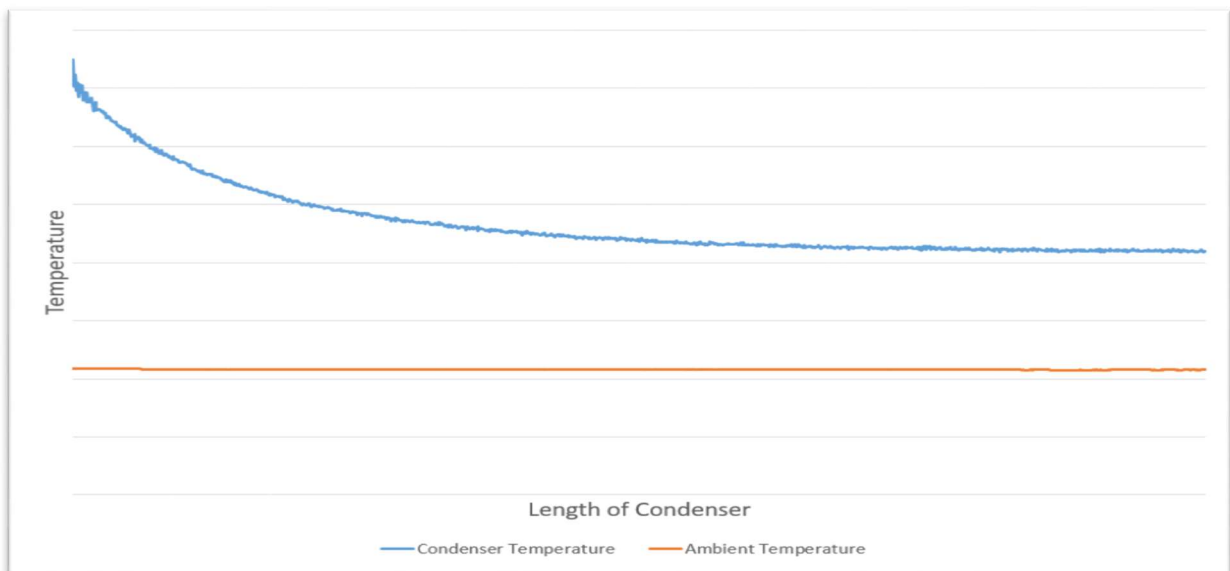
Figure 3.5 Temperature Distribution of Refrigerant along condenser length
