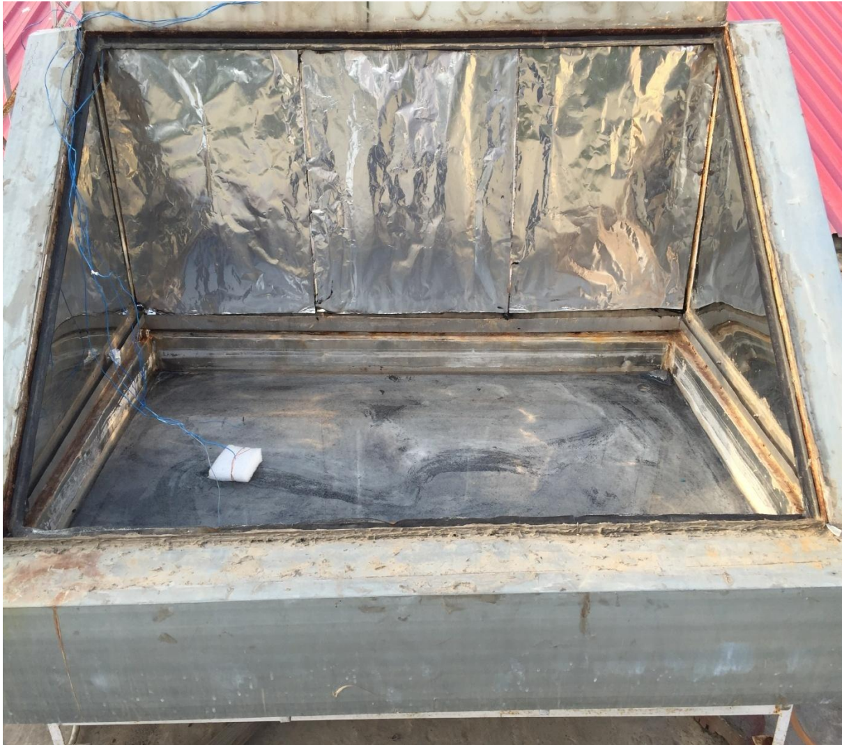
Figure 3.2. Reflectors on sidewalls and back plate
