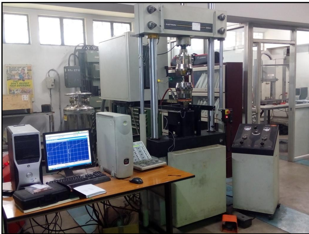
Figure 3.12 Tensile testing machine used in the present work (Courtesy: NML, Jamshedpur).
