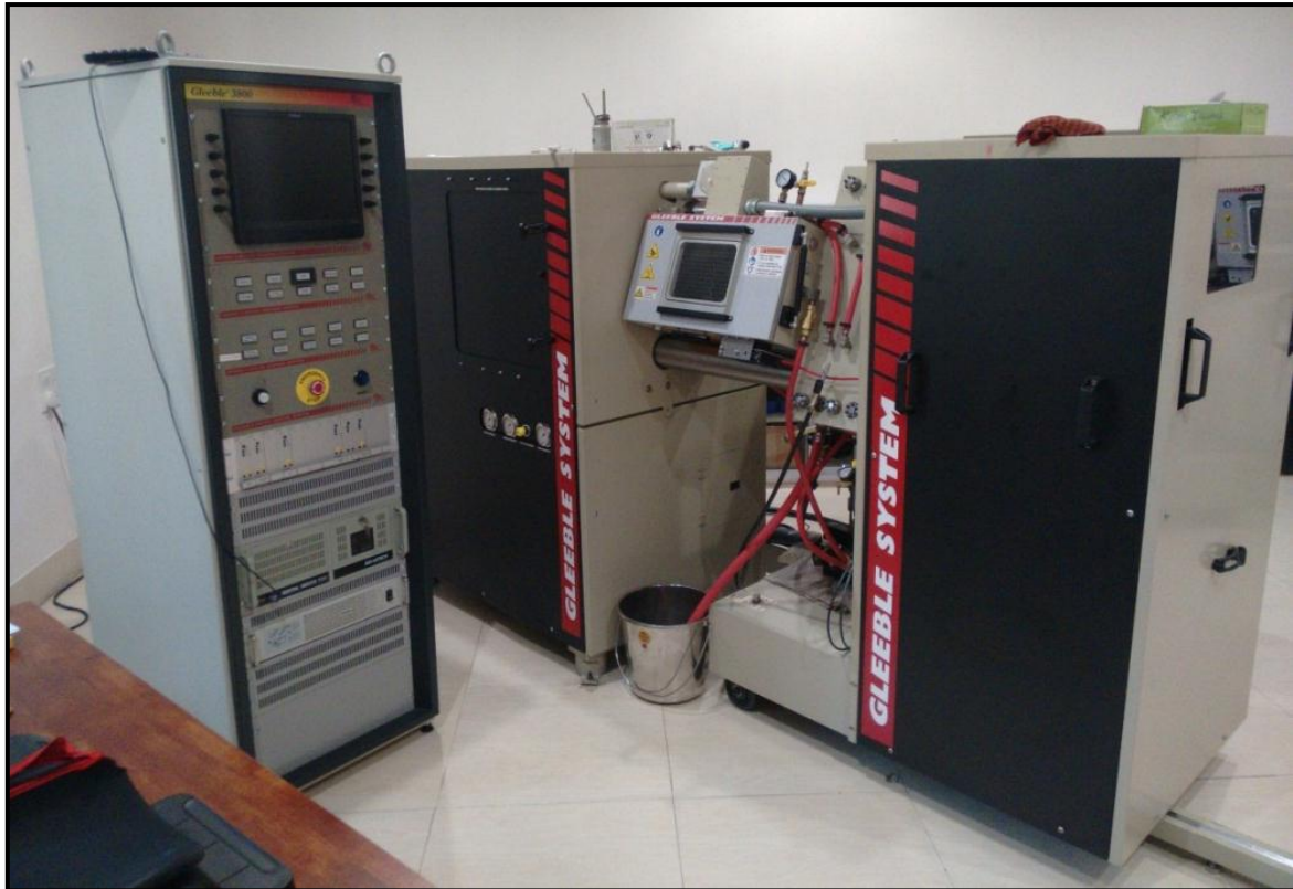
Figure 3.5 Gleeble 3800 simulator (Courtesy: NML, Jamshedpur).
