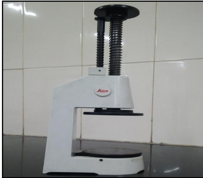
Figure 3.8 Levelling machine (Courtesy: NML, Jamshedpur).
