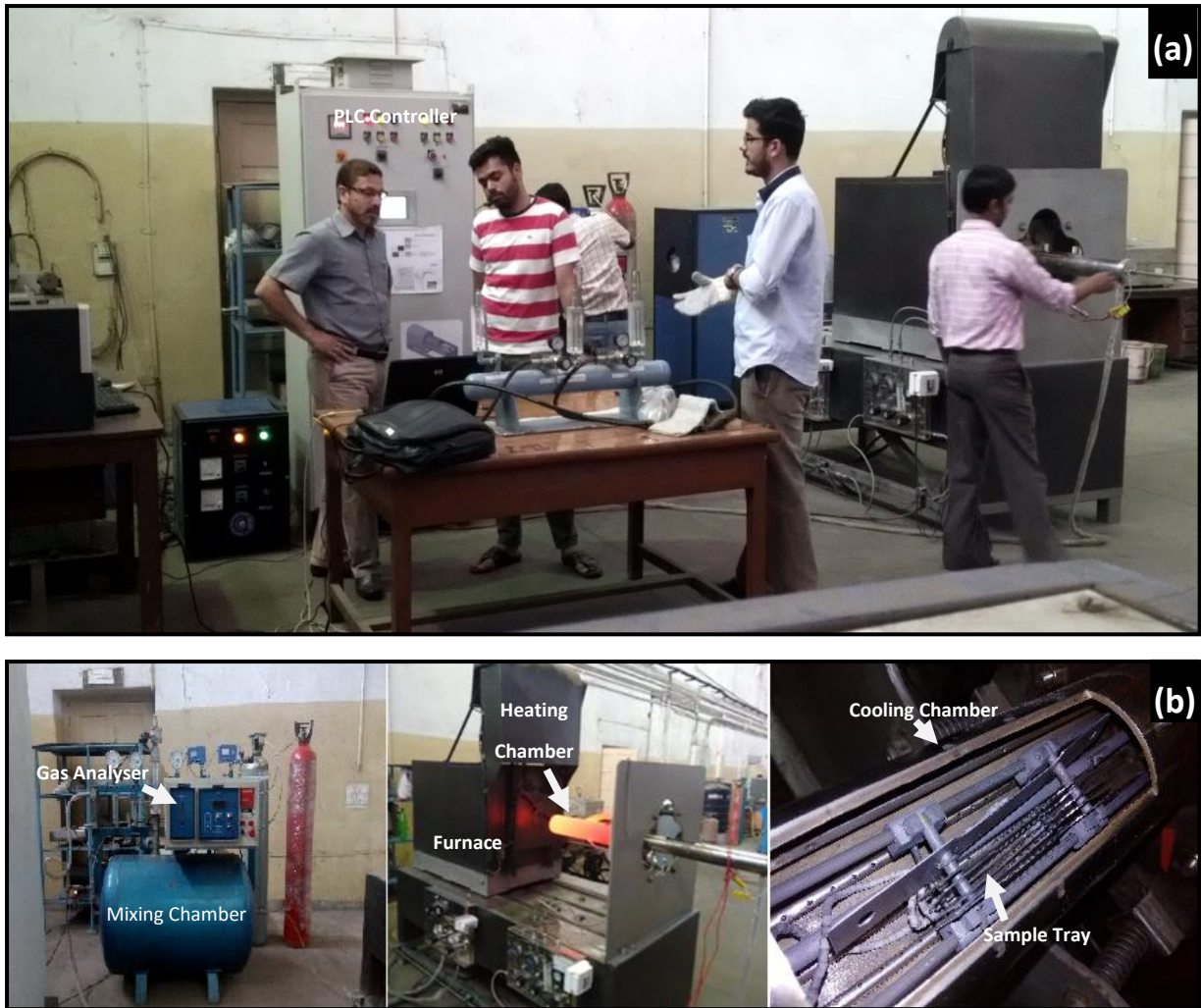
Figure 3.4 Annealing simulator (a) during the annealing process, (b) section details (Courtesy: NML, Jamshedpur).
