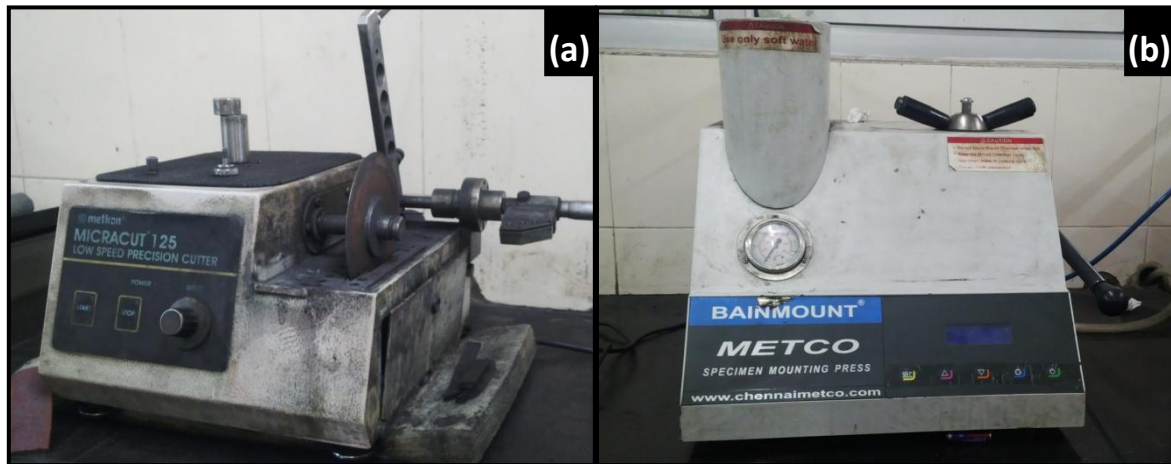
Figure 3.6 (a) Low speed precision cutter, (b) mounting machine (Courtesy: NML, Jamshedpur).
