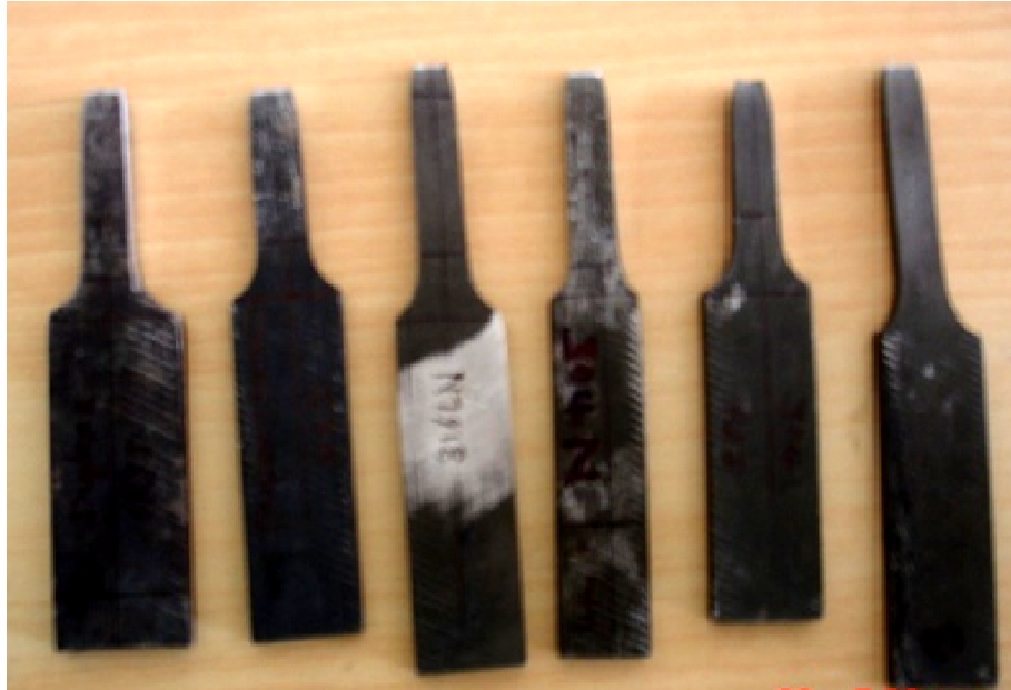
Figure 4.9: Tensile tested samples.
