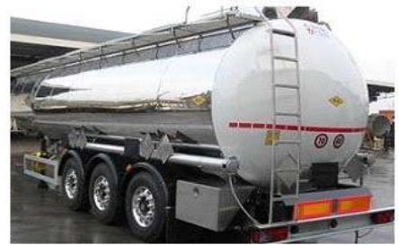
A bitumen road tanker manufactured from LDX2101
