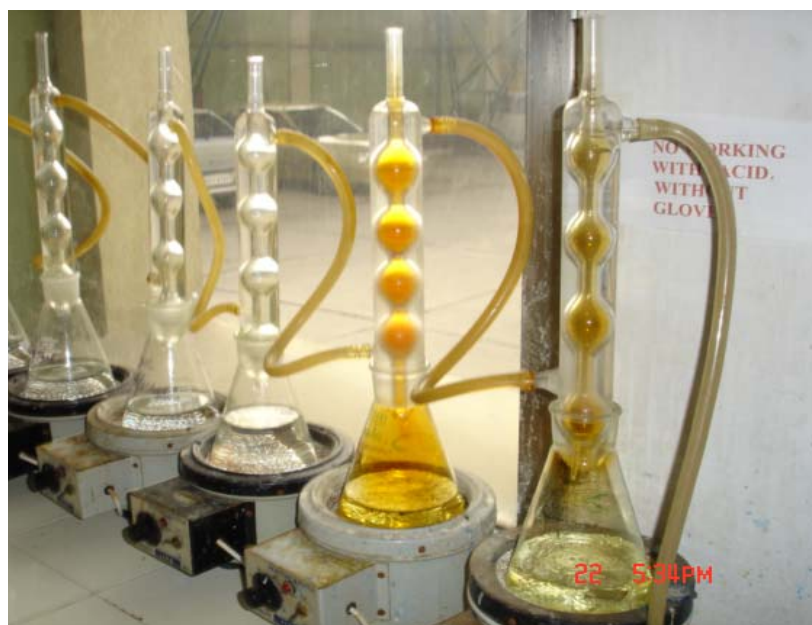
Figure 3.8: Setup corrosion testing in boiling media.
