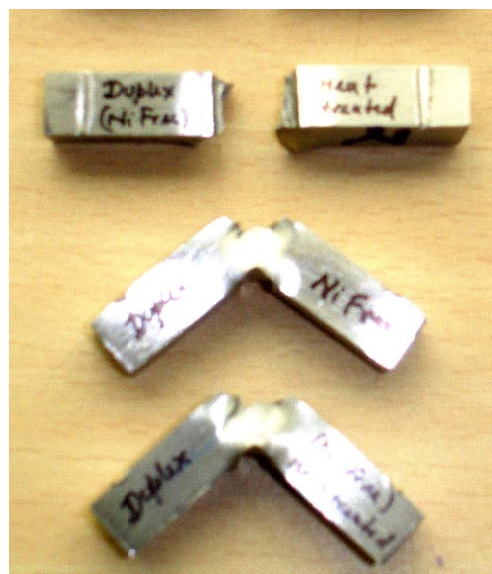
Figure 4.10: Impact tested samples.
