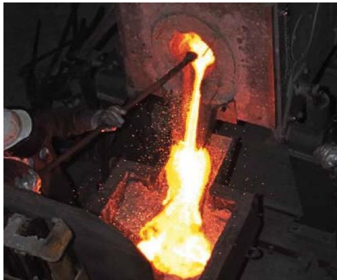
Figure 3.2: Melting of alloy in 100 kg Induction Furnace.
