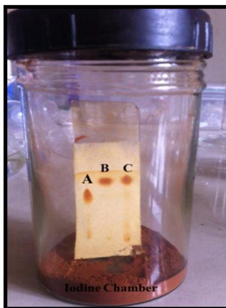
Figure 4.5 TLC analysis of (A) waste cooking oil, (B) waste cooking oil derived methyl ester and (C) methyl oleate standard
