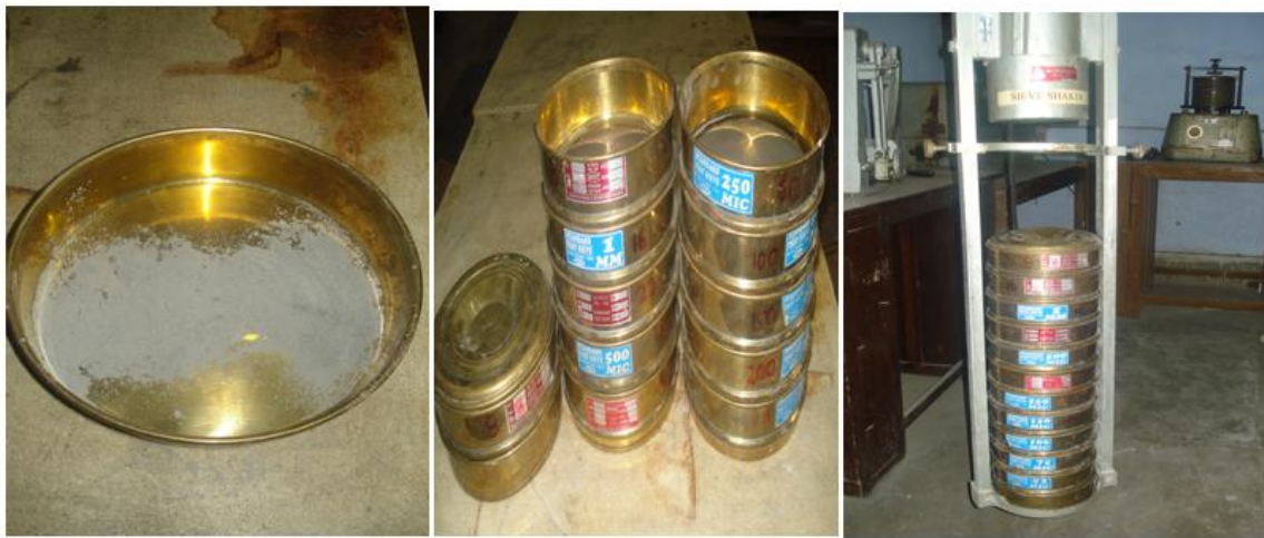
Figure 3.2.2 (a) Fly ash sample (b) Sieve system arrangement (c) Mechanical sieving machine
