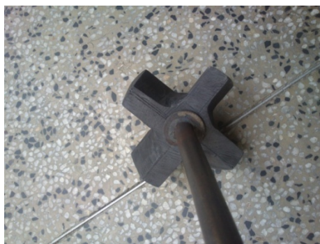
Figure 3.3 Designed Graphite stirrer
