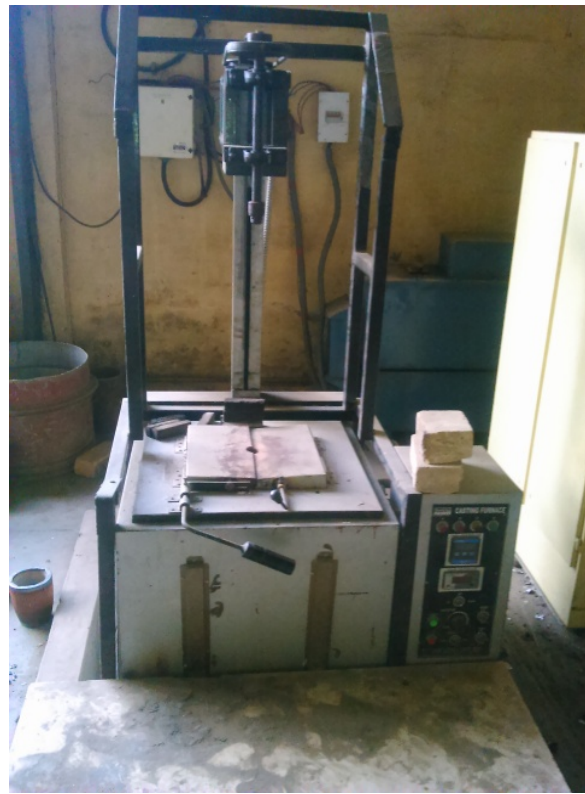
Figure 1.1 Stir Casting Furnace [Photo courtesy: Thapar university campus, Patiala]
