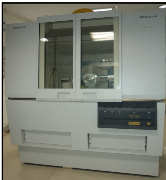
Figure 3.8: X-Ray Diffractometer (Photo courtesy: SAI Labs, Thapar Technology Campus, Patiala)
