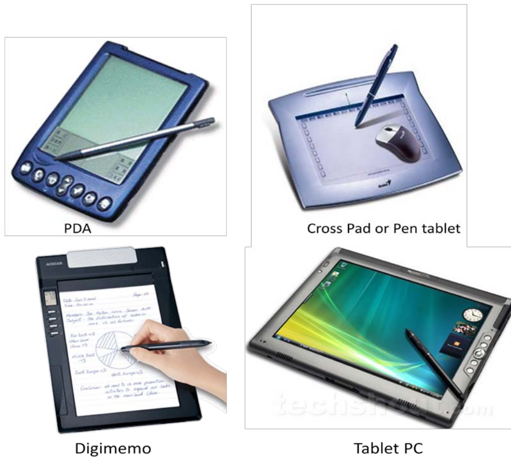
Fig. 2.2: Commonly used hardware devices for capturing handwriting.
