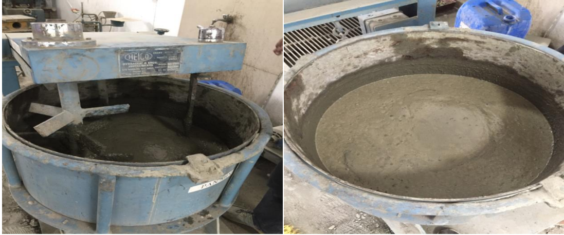
Fig. 3.9: Mixing of Constituents of SCC in a Pan Mixture
