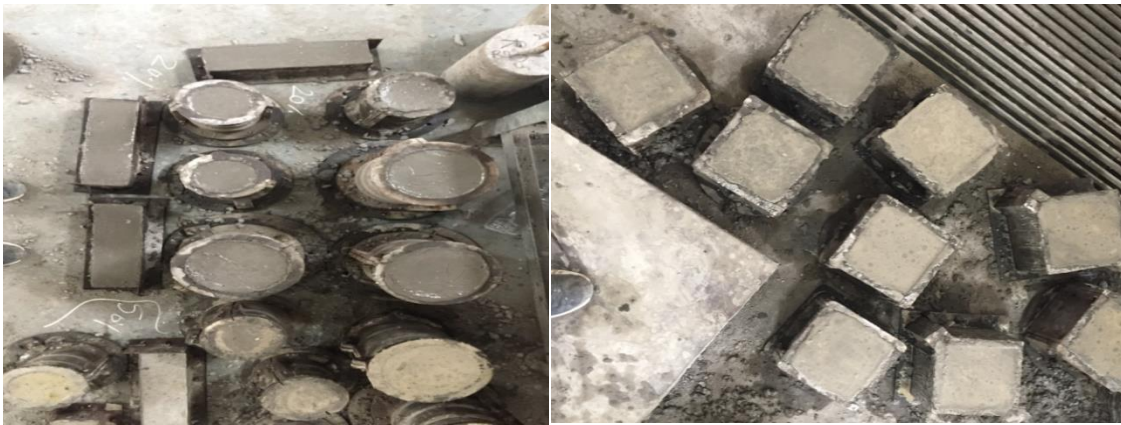
Fig. 3.10: Casting of SCC Samples
