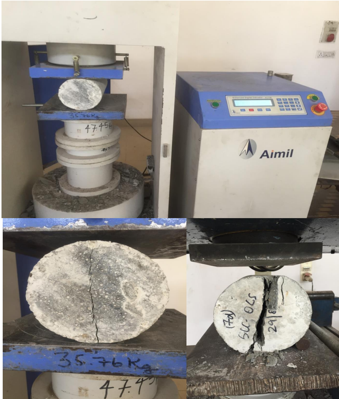
Fig. 3.17: Splitting Tensile Strength Test
