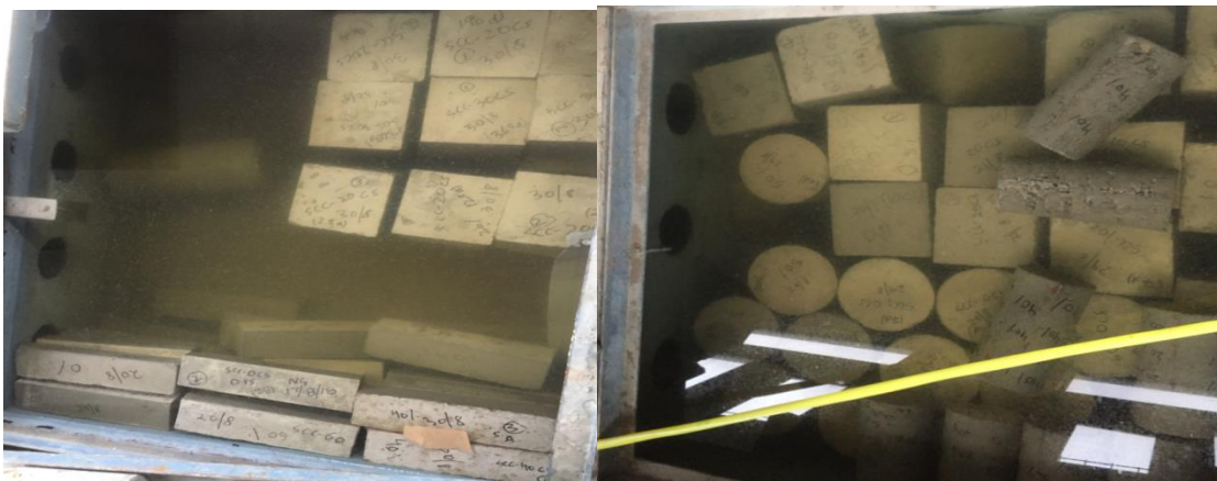
Fig. 3.11: Curing of SCC Samples
