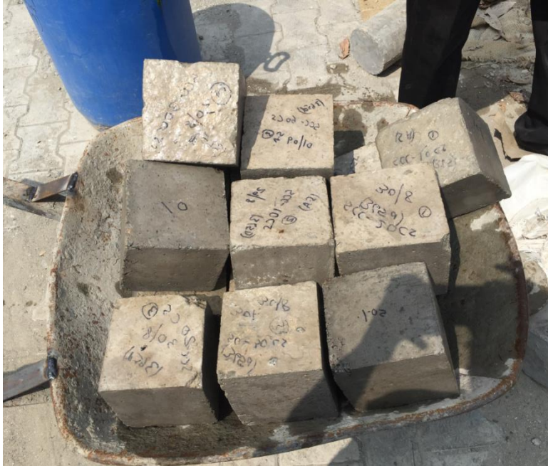
Fig. 3.23: SCC Samples (150 mm Cubes) for Sulfate Resistance Test
