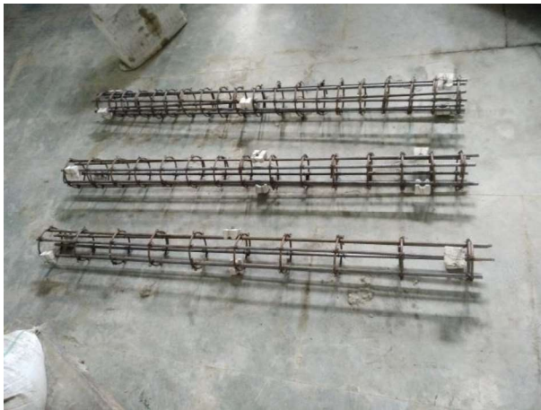
Fig 4.10: Reinforced sections with concrete cover
