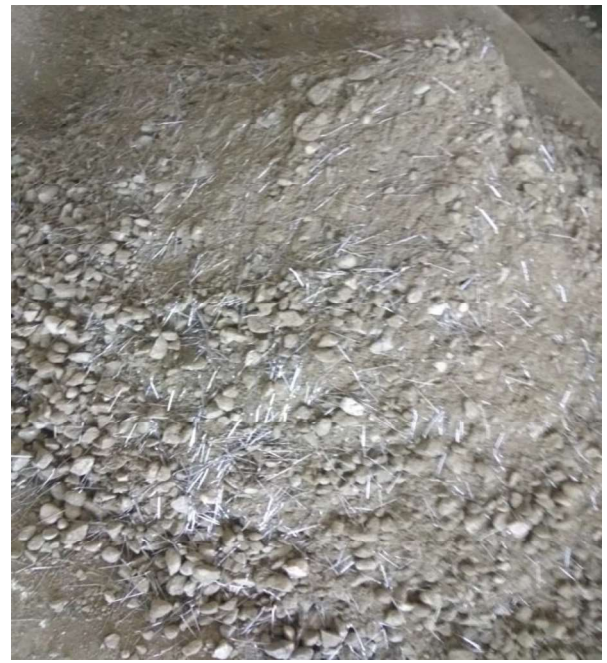
Fig 4.13: Dry mix of the steel fibres
