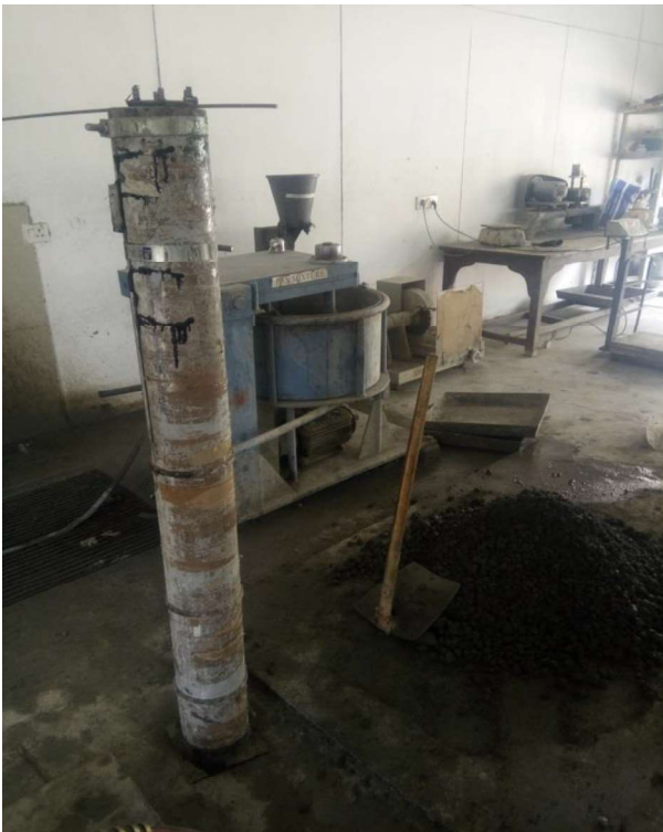
Fig 4.14: Concrete placing inside the mould
