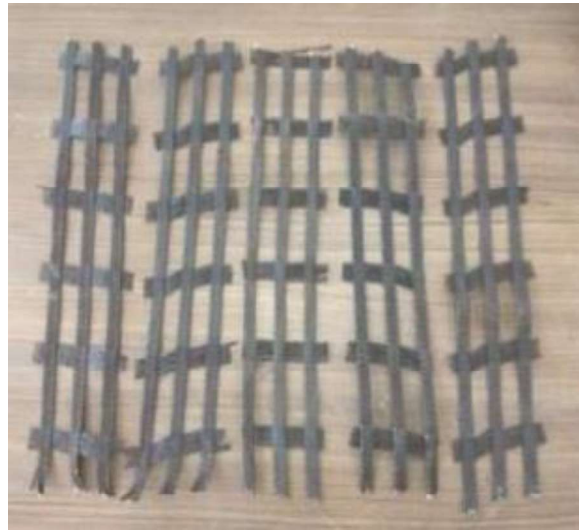
Fig 4.6: Geogrids strip after cutting to required length and width
