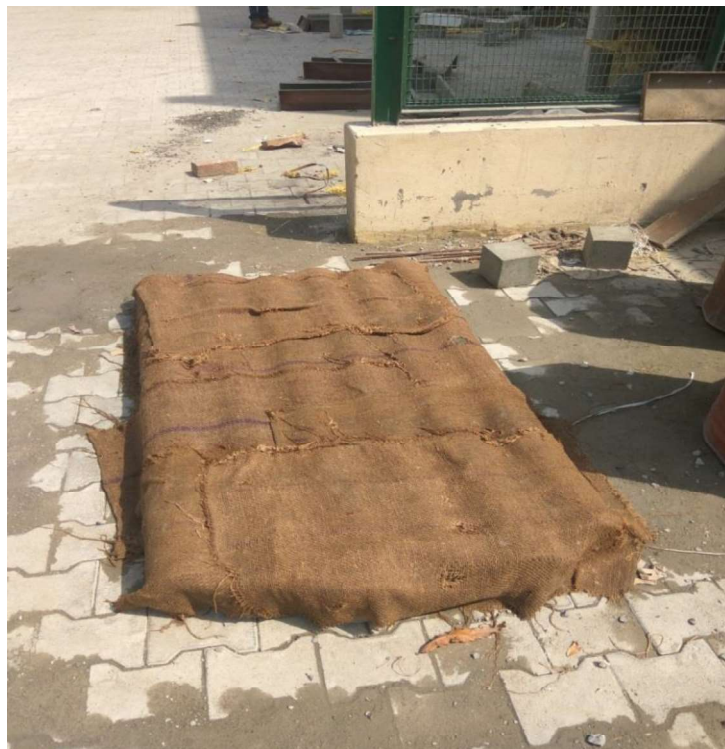
Fig 4.17: Curing circular specimens with jute sacks placed over it
