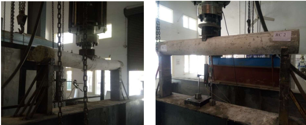
Fig 4.18: Experimental setup for shear testing
