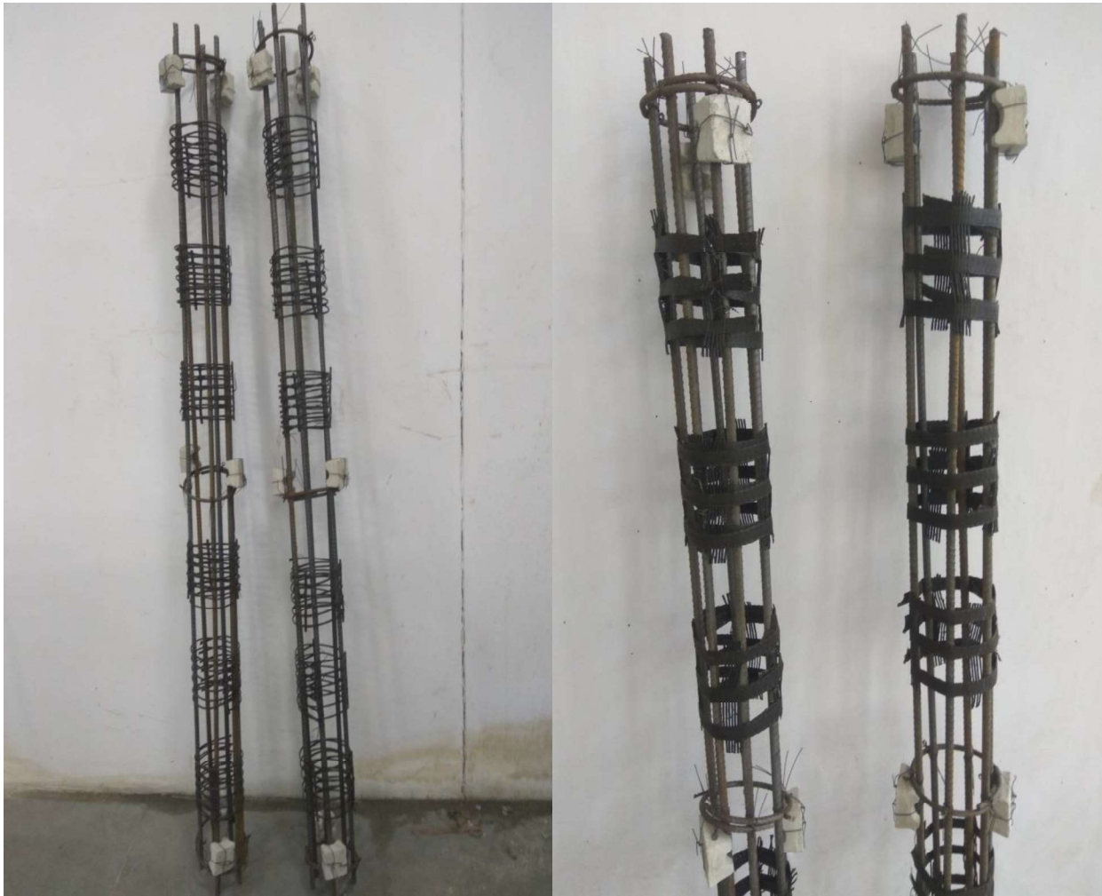
Fig 4.9: Applying geogrids for 700 mm stirrups spacing
