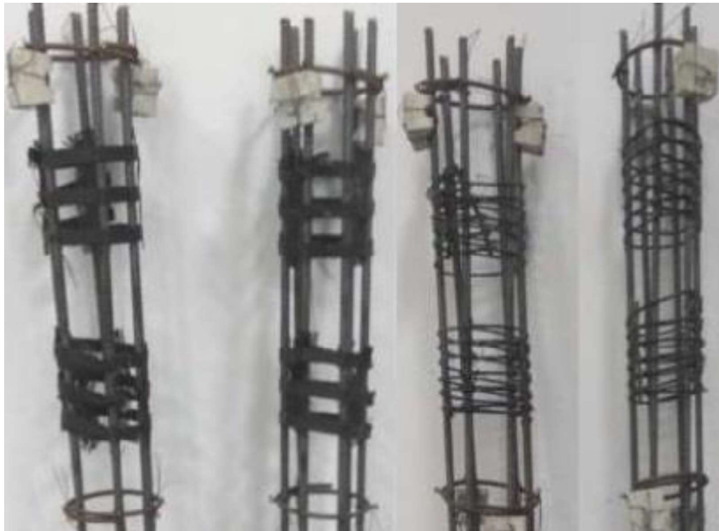
Fig 4.8: Applying geogrids for 450 mm stirrups spacing
