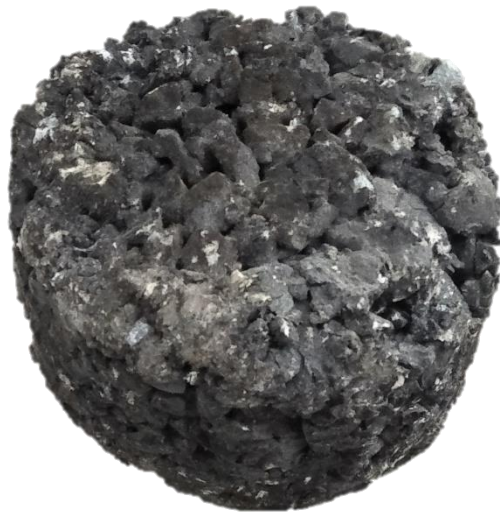
Figure 4.4 Sample of OGFC Mix obtained after Cantabro Abrasion Test
