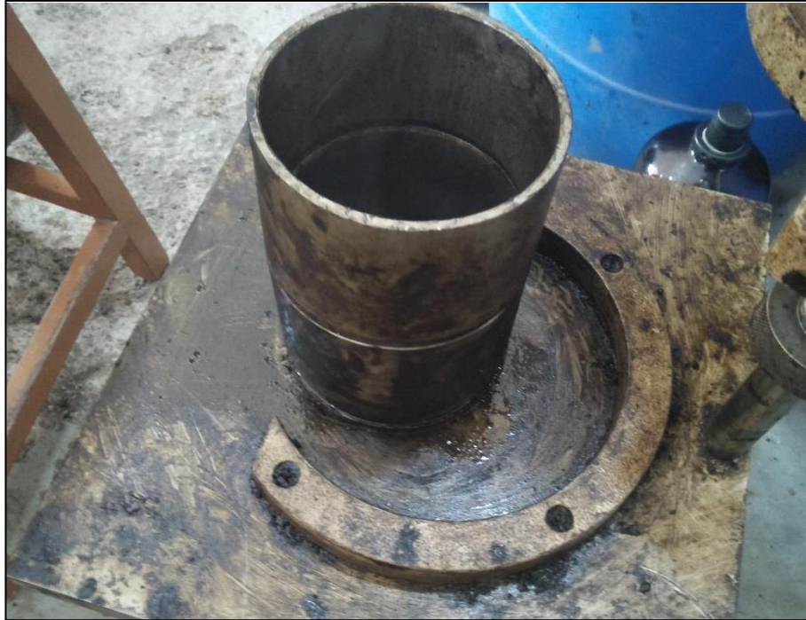
Figure 3.6 Marshall Mould Arranged with Collar and Base Plate
