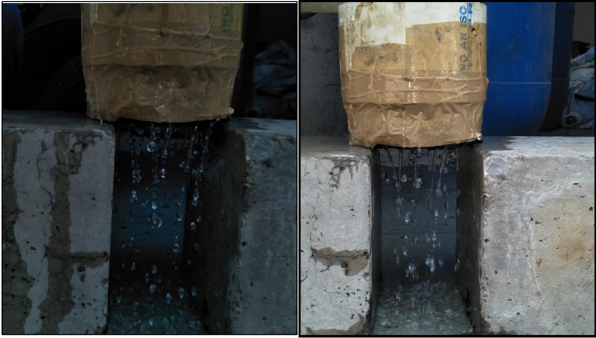
Figure 3.15 Water Percolate through the OGFC Mix sample
