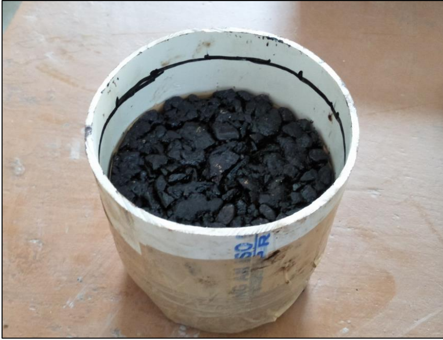
Figure 3.13 Marshall Mix Sample Fixed with Pipe
