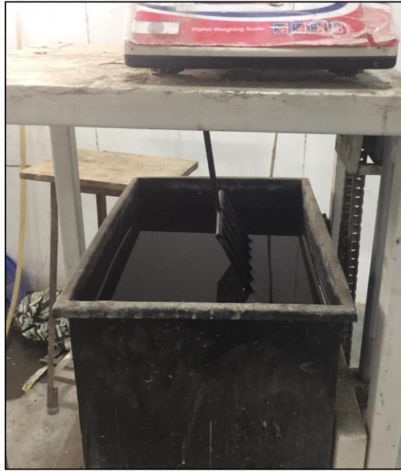
Figure 3.10 Noted the Weight of Sample Suspending in Water
