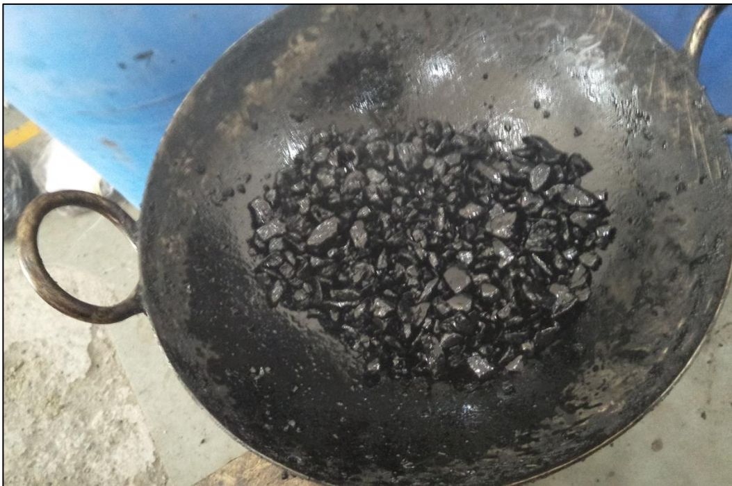
Figure 3.5 Mixing of Aggregates with Binder
