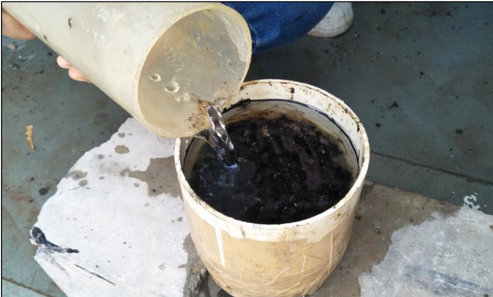
Figure 3.14 Water Maintained for Constant Head
