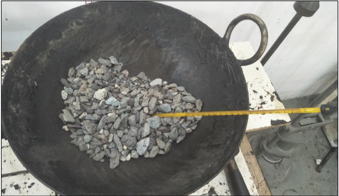
Figure 3.4 Shows the Aggregates heated to Obtained the Required Temperature.
