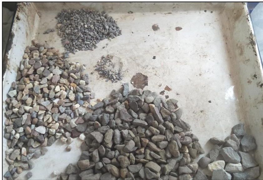
Figure 3.3 Shows the Different Size of Aggregates used as per the Gradation (NAPA IS-115)
