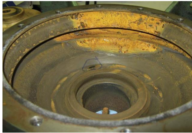
Figure 1.1. Erosion wear on casing of centrifugal pump at actual condition [Noon and Kim, 2016, Electronic and printing permission of ©Elsevier].
