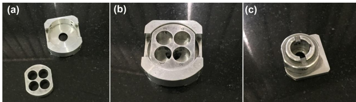
Figure 3.4. (a & b) Multiple sample and (c) single sample holder for SEM of powdered samples.
