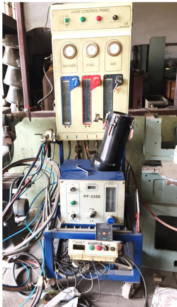
Figure 5.4. HVOF spraying unit [Harsha Specialty Welding and Coatings, Panchkula, India].
