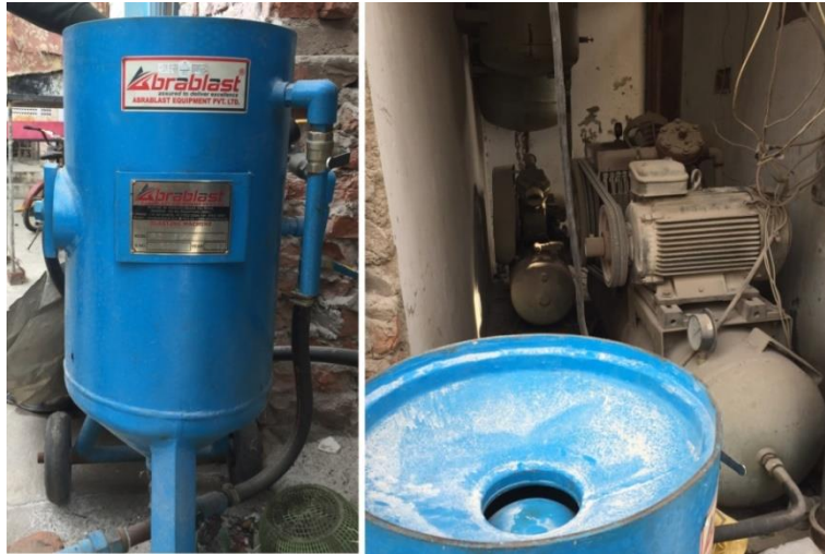
Figure 5.3. Sand blasting unit [Harsha Specialty Welding and Coatings, Panchkula, India].
