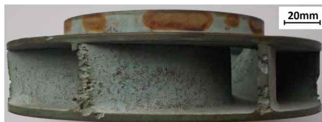
Figure 1.3. Cavitation erosion wear on radial impeller at actual condition (Szala et al. 2014).
