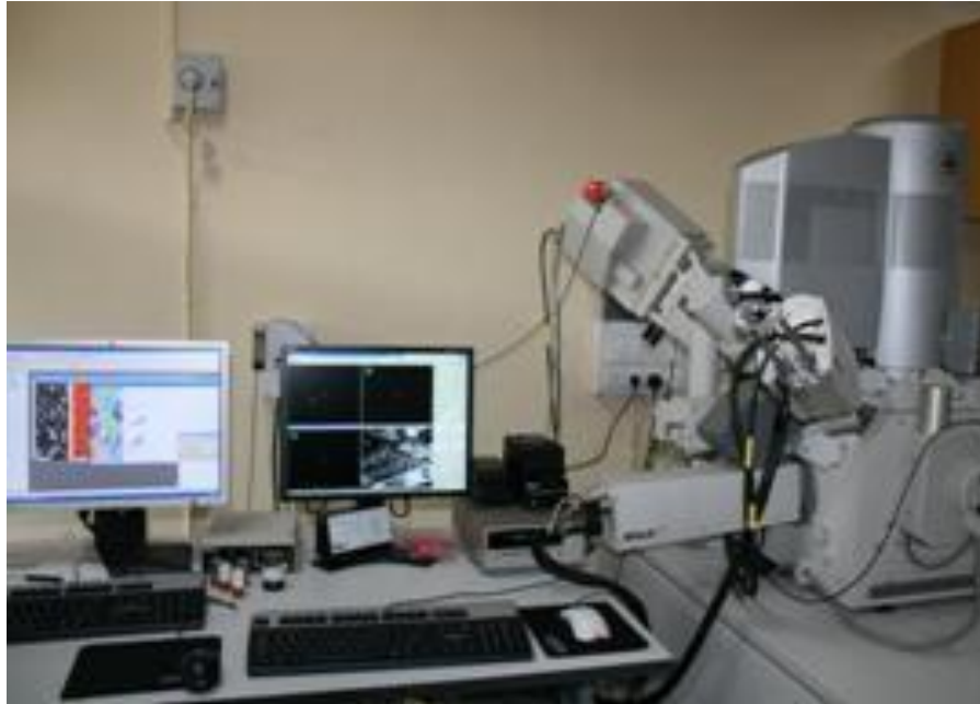
Fig 4.4 Fie Quanta 3D FEG Electron back-scatter diffraction apparatus (Courtesy: Department of Metallurgical Engineering & Materials Science, IIT Bombay)
