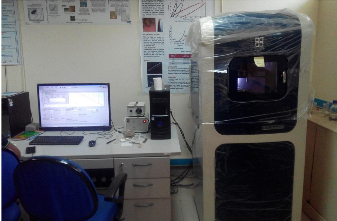
Fig 4.5 Nanomechanical Test Instrument, HYSITRON Inc, USA (Courtesy: NanoIndentation Lab, IIT Ropar, Punjab)
