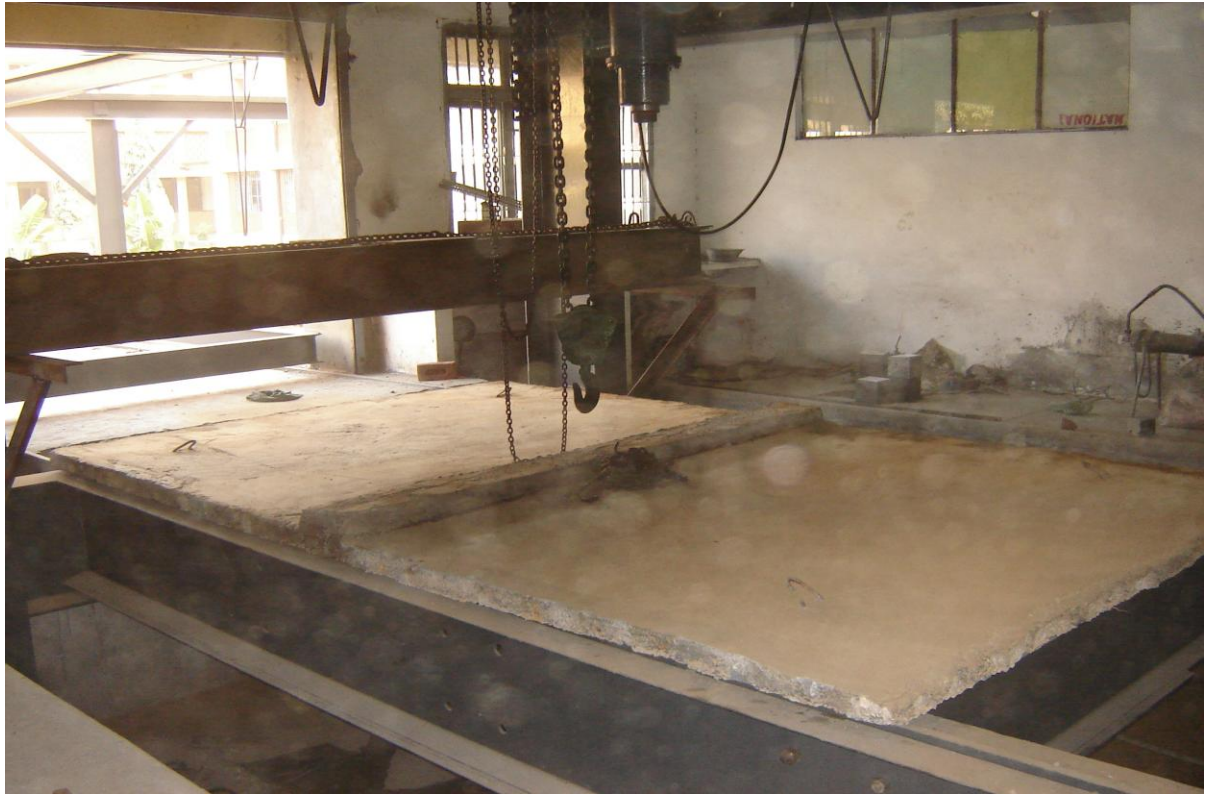
Figure 4.11: Typical Schematic Diagram showing the placement of Slab in Reaction Frame
