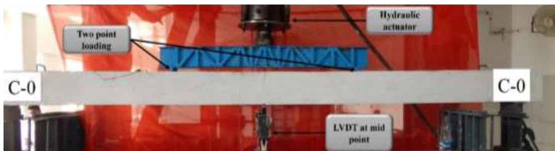
Figure. 3.15. Flexure testing set up
