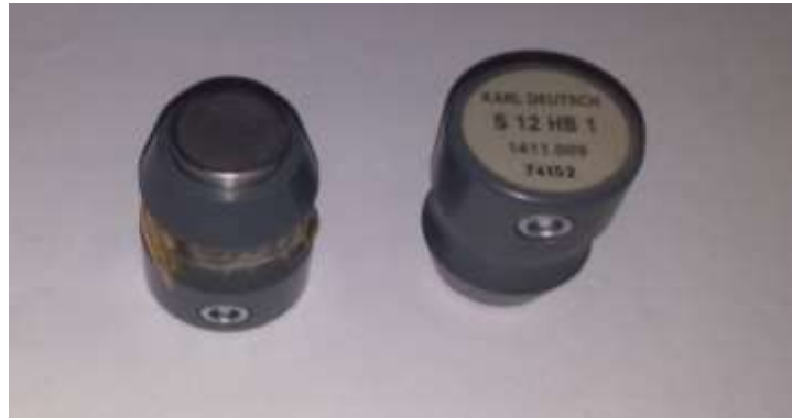
(a) Transducer (S12 HB 1) (12 mm diameter) of 1 MHz frequency
