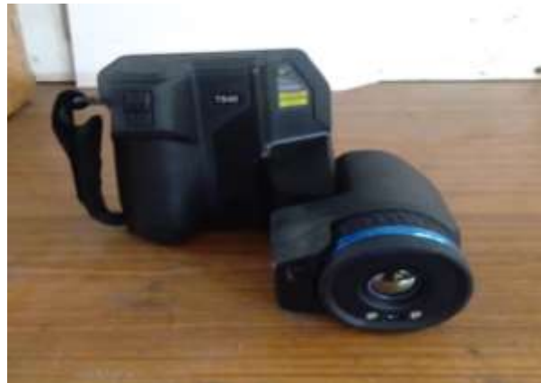
(a) FLIR T-540 used in study
