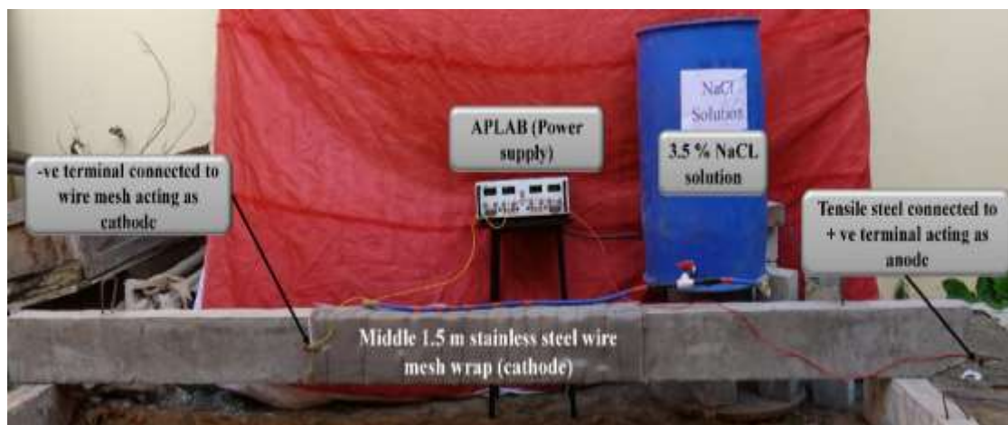
Figure 3.12. Accelerated impressed current corrosion set up
