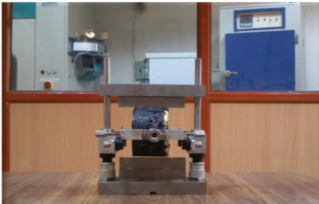
Photo 3.10: Apparatus for Resilient Modulus Test
