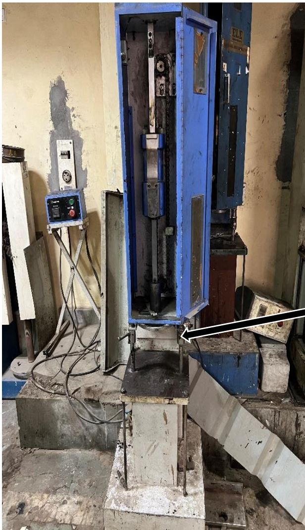
Photo 4.2: Marshall compactor for compaction specimen at mix design stage.
