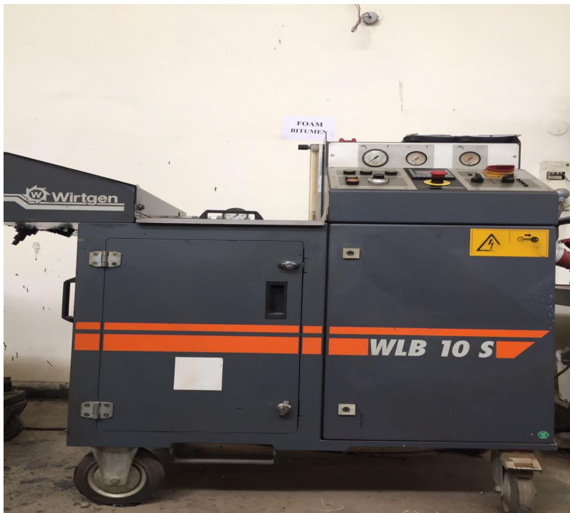
Photo 3.6. Foaming plant (WLB 10S) used for the present study
