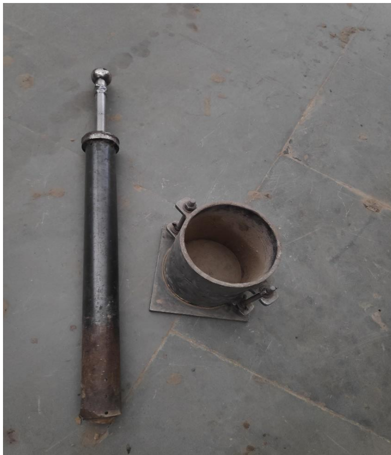
Photo 3.8: Apparatus for modified proctor test
