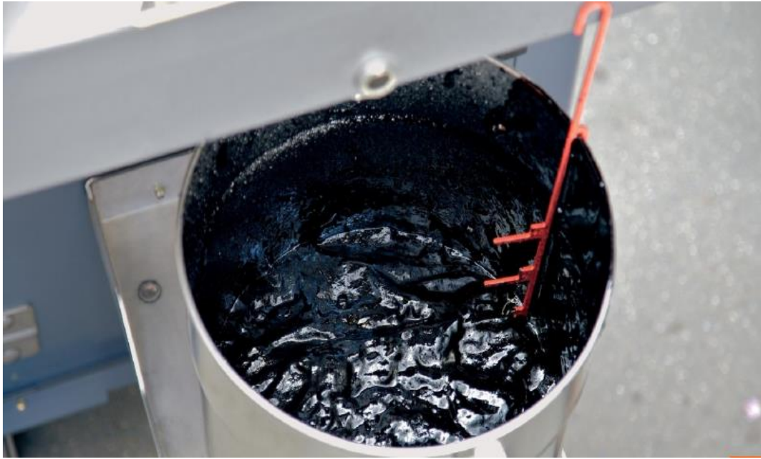
Photo 3.7: Dipstick supplied with Wirtgen WLB 10 S
