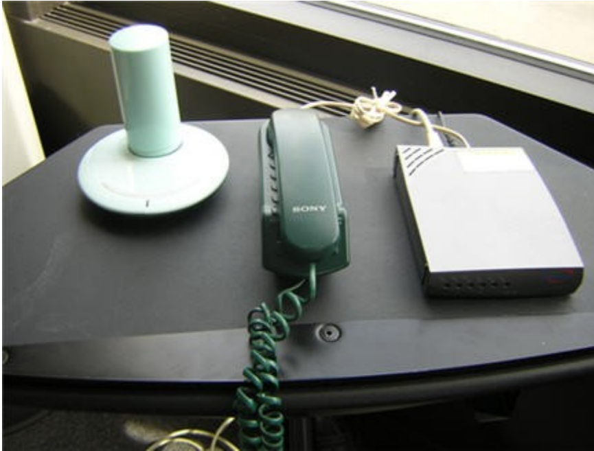
Figure 1.6: Indoor WiMAX CPE (Airspar EasyST) - object on left) [9]
