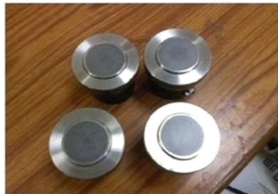
Fig. 4.7: Contact type transducers (Karl Deutsch Make)
