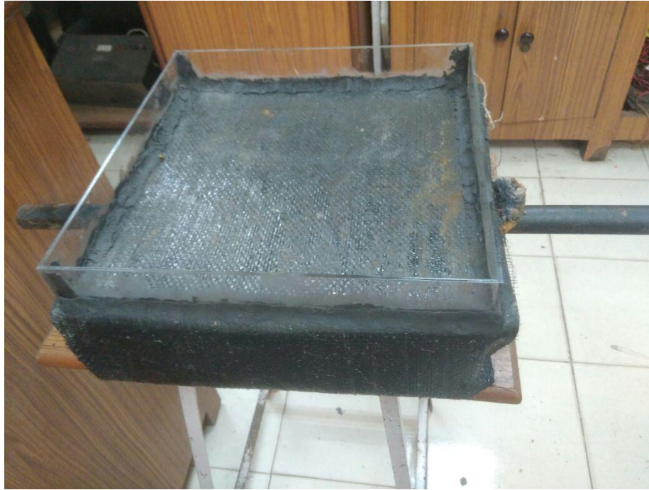
Fig. 4.4: Slab specimen wrapped with CFRP
