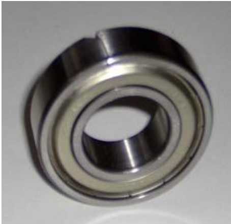
Figure 4.3: Crank in the outer race
