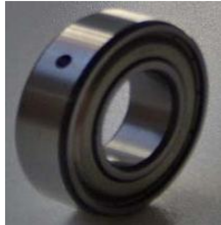
Figure 4.4: hole in the Outer race
