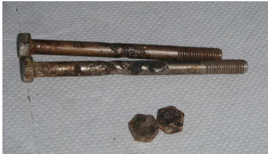
Fig. 2.6 Bolt and screw corroded due to Crevice corrosion ( Autolab application note 16 )
