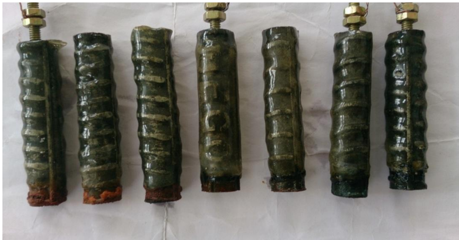
Plate 6.3 – Type 2 steel specimens from 1-7 after corrosion
