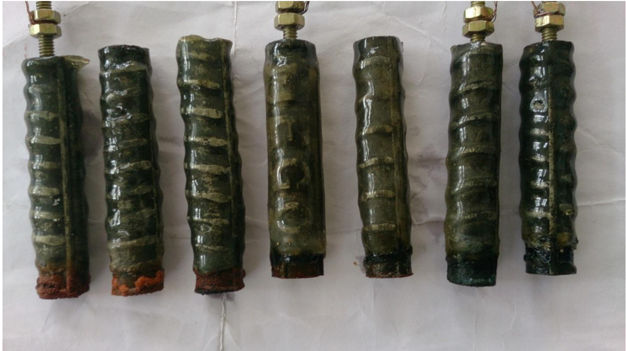
Plate 5.6 – Condition of steel rebars of Type 2 test series at the end of test
