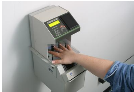
Figure 15 Hand geometry scanner
