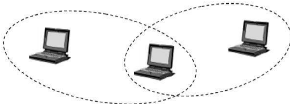
Figure 1.4 Example of a Wireless Adhoc Network
