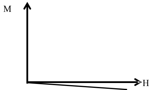
Figure 1.2: M vs. H curve for a diamagnetic material [7].
