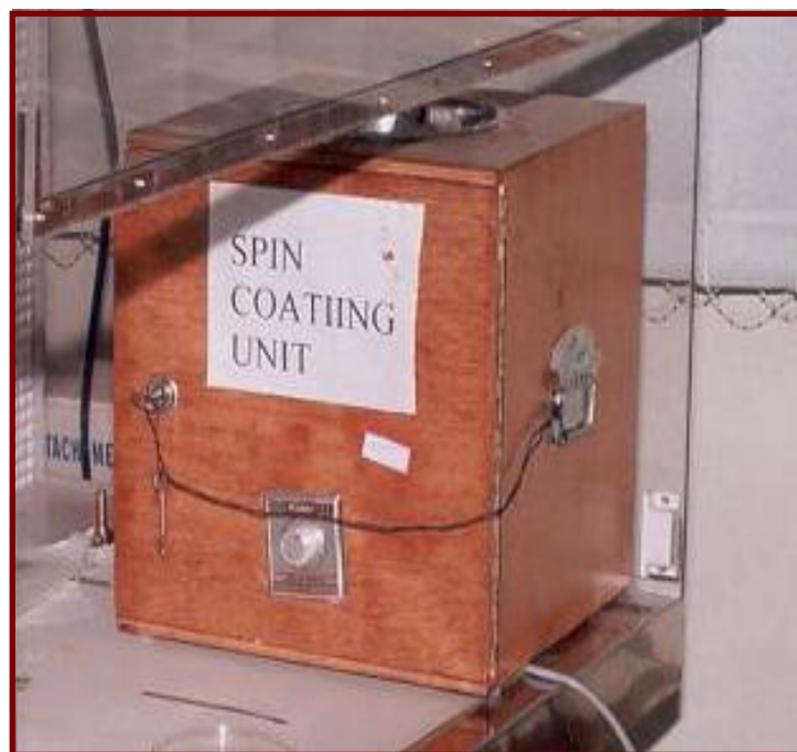
Figure 3.4 Spin coating unit for polymer coating of glass substrates.
