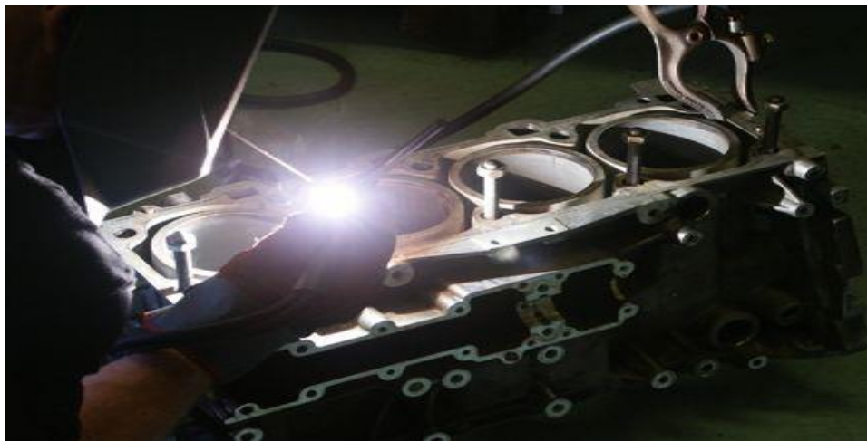
Figure 1.4: Welding inside cylinder to fill the required material [29]
