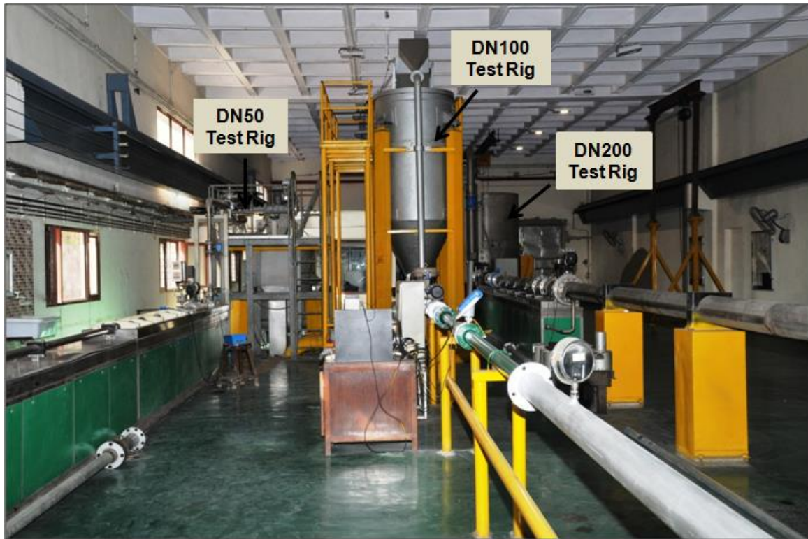
Figure 3.18: Complete DN100 Test Rig. Also shown are DN50 and DN200.
