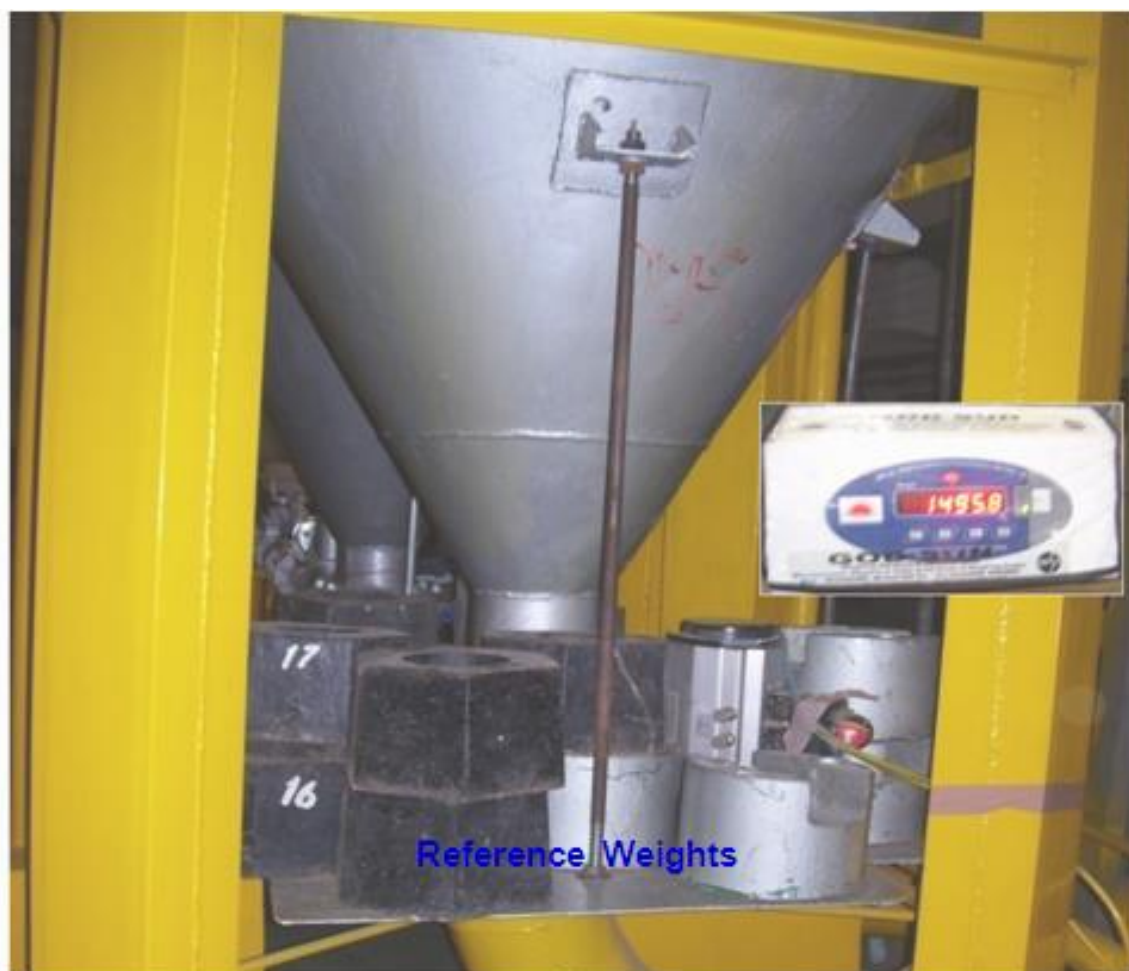
Figure 4.1: Calibration of the weighing system using reference mass standards.
