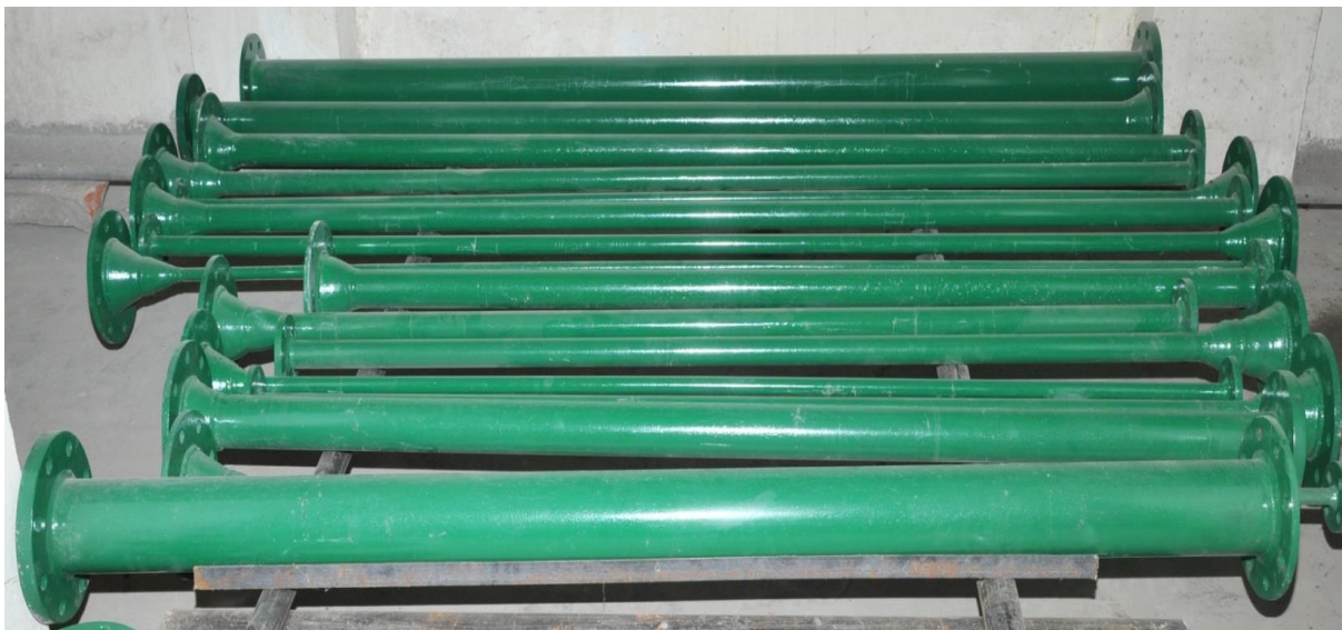
Figure 4.11: Adaptors of (15-100) mm sizes fabricated from seamless MS pipe.
